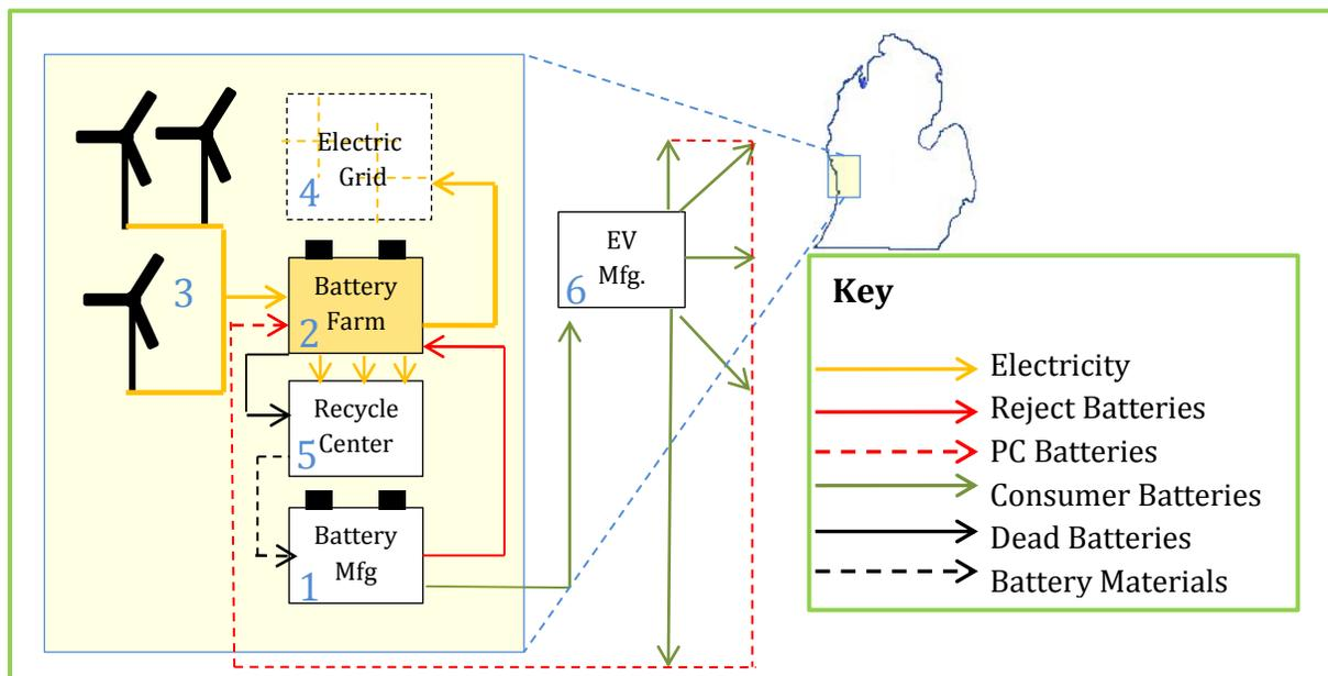
**Figure 1: Flow Diagram - EV Battery Wind Storage System**
