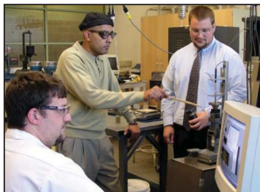
In a senior design project that seeks to improve quality in foundry processes involving green sand, MFT senior Ron Davis (seated) monitors the vibration results of cone-jolt testing done on a two-inch specimen of sand being tested by Dr. Sam Ramrattan , project advisor, and MFT senior Mike Horvath . The third member of the project is UEM senior Alex Hiday . The project will be presented at the 43rd Conference on SEDP at 9:30 a.m. in Parkview Room D-201.
