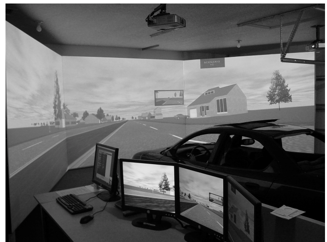
Figure 1. Picture of 180 field of view STISM M500W™ simulator with integrated car cab and control station.
