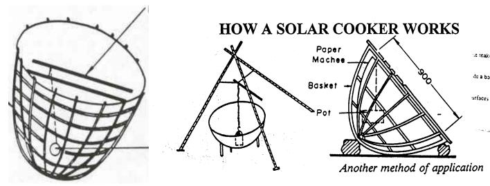
Fig. 1. Illustrative view of the solar cooker, and its application
