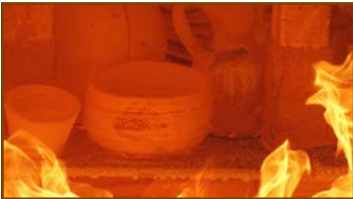
Temperatures in the wood-fired kiln reach 2400 degrees Fahrenheit
