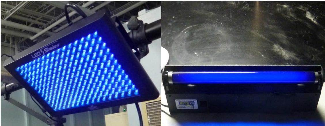
**Figure 4.5** UV excitation sources (from left to right) – UV LED array, blacklight lamp
