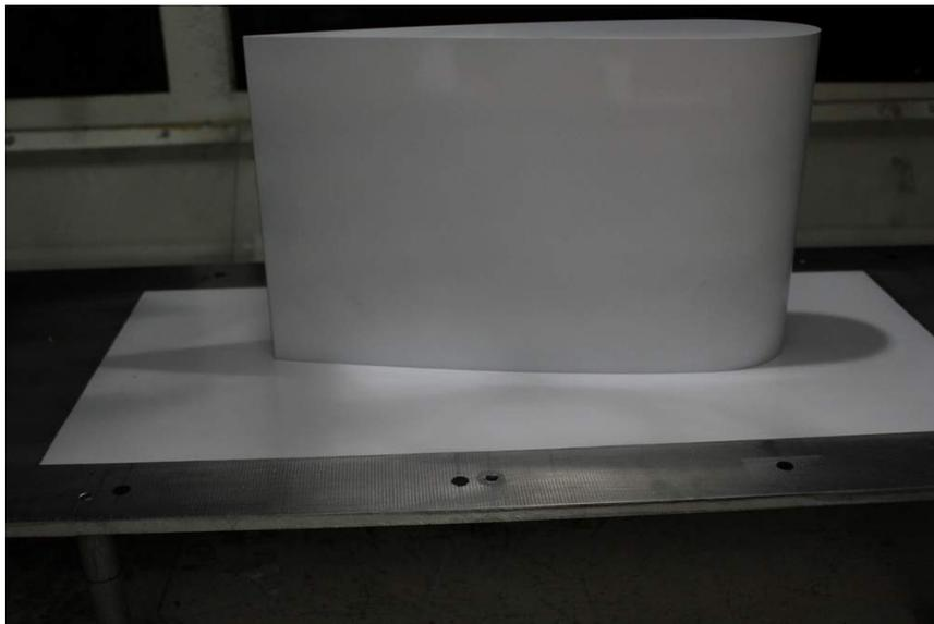
**Figure 8.2** Rood wing mounted on an elevated flat plate in the wind tunnel test section
