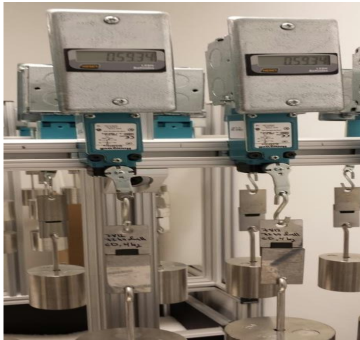
Figure 3.1: Static Shear Test Lab Setup
