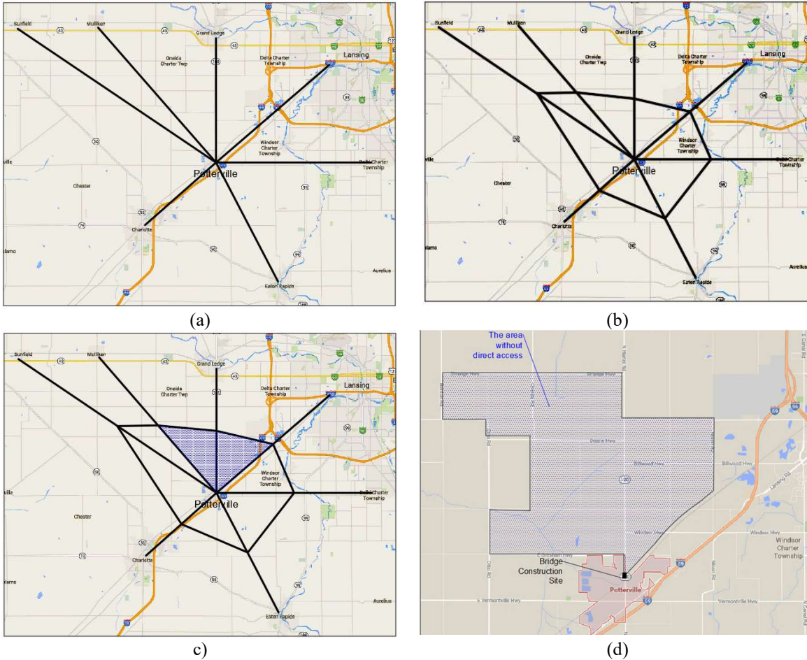
Figure 10. Steps taken to establish the area without direct access during construction
