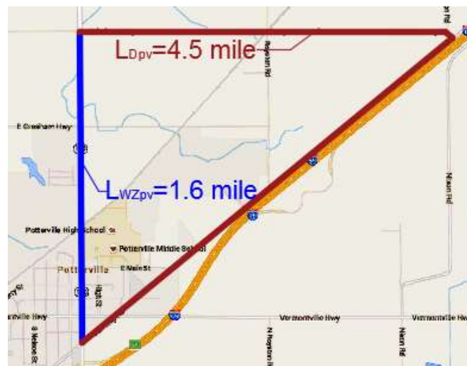
Figure 6. Length of detour, and road segment closed during construction for passenger vehicles
