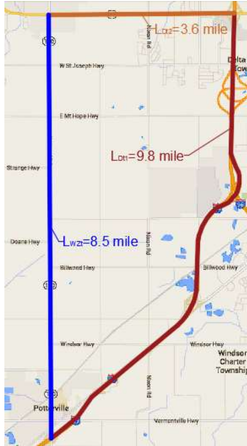
Figure 7. Length of detour, and road segment closed during construction for trucks
