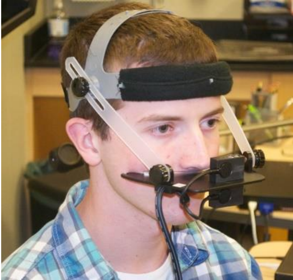
Figure 3. Nasometer II 6450 headset with plastic seal in typical configuration above upper lip on male participant.
