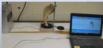
Figure 2. Scanning acetabulum with NextEngine 3D scanner
