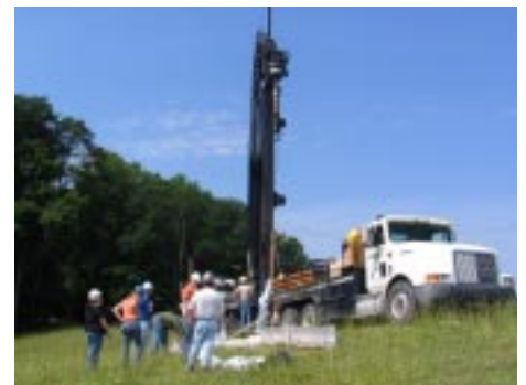
Glacial geology class students describing core during Rotasonic drilling on an esker in Barry County.
