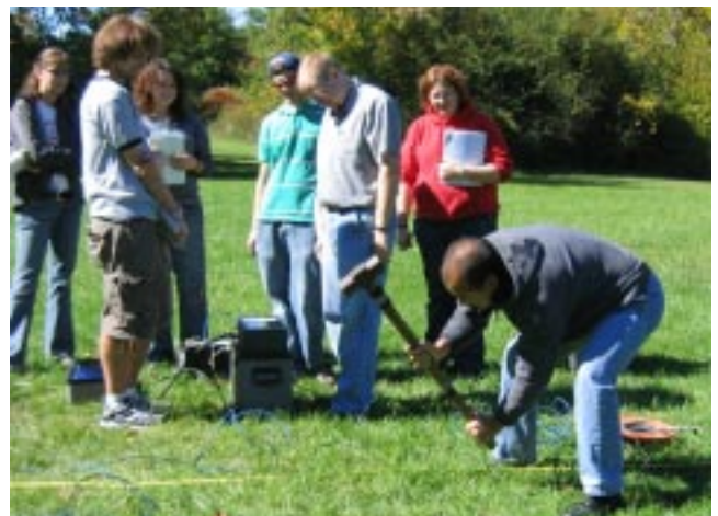
2006 Geophysics Class running a seismic refraction survey.
