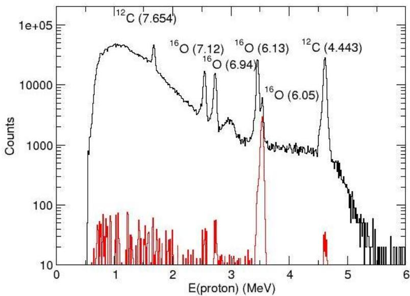
Figure 2. Proton-energy spectra measured in HELIOS from  $^{16}\text{O}(p,p')^{16}\text{O}^*$  inelastic scattering for proton singles (black) and coincidences with  $e^+e^-$  (red). The  $0^+$  excited state of  $^{16}\text{O}$  stands out clearly in the coincidence spectrum. Peaks from a  $^{12}\text{C}$  impurity in the target are also indicated.
