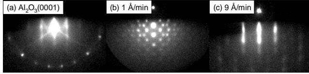
**FIG. 1.** The reflection high energy electron diffraction (RHEED) patterns collected from (a) a clean  $\text{Al}_2\text{O}_3(0001)$  surface and following  $\text{CeO}_2$  growth on  $\text{Al}_2\text{O}_3(0001)$  at  $\sim 650^\circ\text{C}$  under  $\sim 2.0 \times 10^{-5}$  Torr of  $\text{O}_2$  plasma for the growth rates of (b) 1  $\text{\AA}/\text{min}$  and (c) 9  $\text{\AA}/\text{min}$ , indicating the 3-D island growth and 2-D layer growth, respectively.
