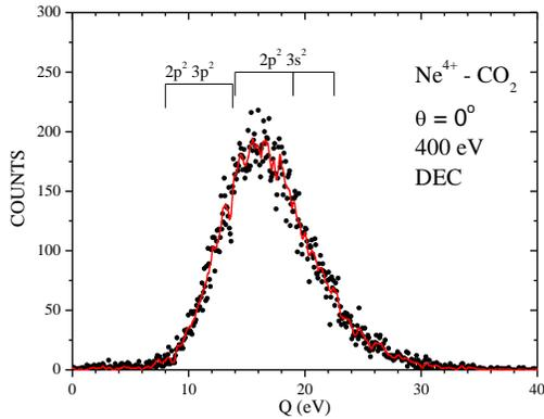
**Figure 3. Translational energy-gain spectrum for double-electron capture by 400 eV  $\text{Ne}^{4+}$  ions from  $\text{CO}_2$  at  $0^\circ$  scattering angle.**
