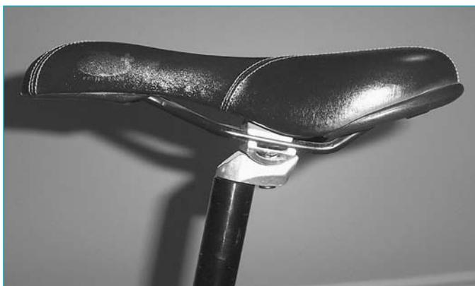
Figure 1 Saddle in a level position.
