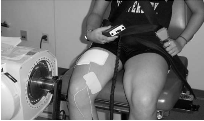
Figure 1 — Position of subject on the Kincom™ Dynamometer with OrthoDx attached to subject.
