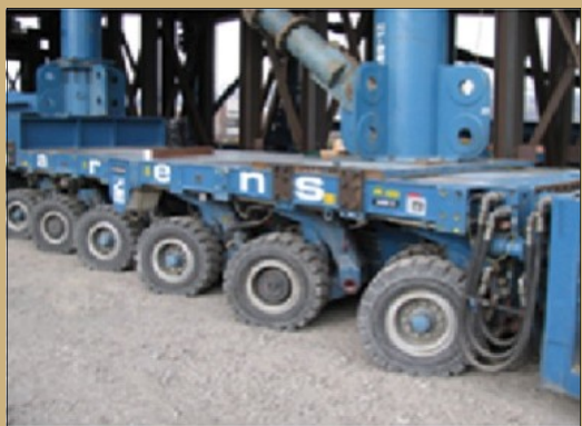
Above: A self-propelled modular transporter (SPMT)
