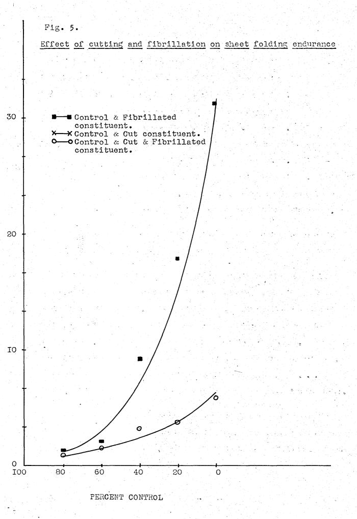
It thus seems clear that the necessary fiber treatment here is that of maximum fibrillation of the long fiber fraction in the pulp. Obviously fiber length is of utmost importance in the fold test as without it the folding endurance of a sheet will be at best, mediocre. It seems essential then, that for optimum folding endurance of any pulp, the fibers making up that pulp be subjected to as little cutting action as possible.
