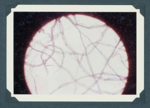
Fig. 9 — Control pulp (Pulp A) — showing raw untreated form of a western softwood sulphite pulp = x 100, f/2.8
