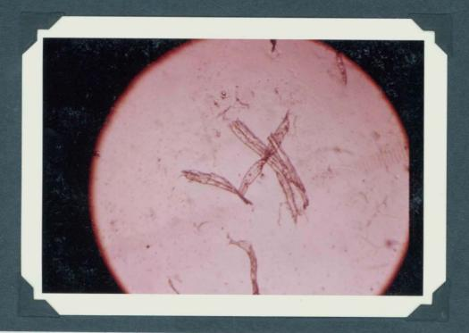
Fig. 10 - Cut constituent (Pulp B) - showing high degree of cutting, with minimum fibrillation development - x100, f/2.8.
