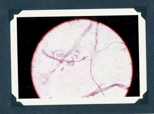
Fig. 11 - Fibrillated constituent (Pulp C) - showing high degree of fibrillation and mucilage formation, with minimum cutting action - x 100, f/2.8.
