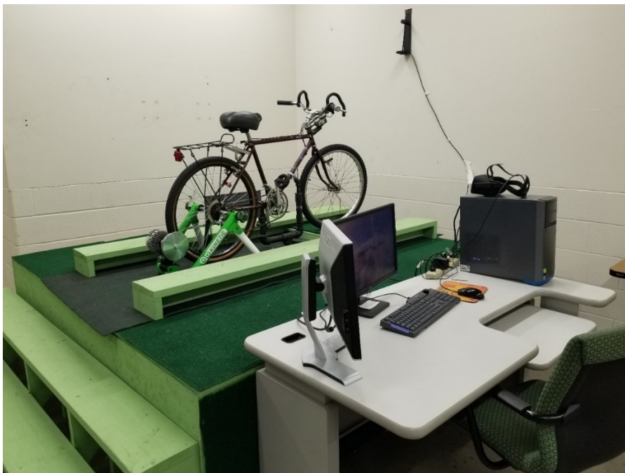
Figure 3.1: Bicycle simulator setup
