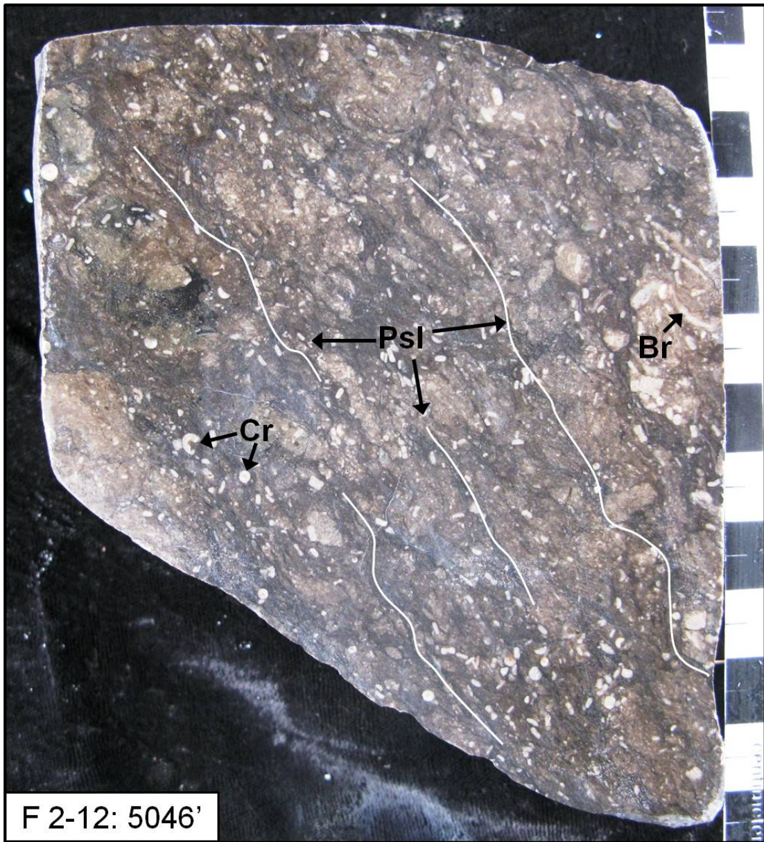
F 2-12: 5046' – Skeletal peloidal packstone-wackestone with grainstone burrow fill (?). Pressure solution/stylolite seams (outlined with white lines) are oriented approximately 50 degrees from horizontal, indicating non-vertical stresses applied to the sample, and/or sample rotation from the original pressure solution development orientation.
