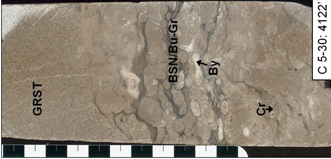
C 5-30: 4122'- F3 - Peloidal-skeletal packstone with grainstone bed (GRST) capping this sample. Burrow-bounding stylonodular fabric with grain-rich burrow fill is prominent in the center of this sample. C 5-30: 4119'- F1/5 - Dark gray/black wackestone-mudstone overlain by beige brachiopod skeletal fragment packstone.
