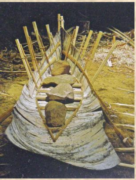
Bending the bark in the canoe building frame. Photo courtesy of R. Nash.
