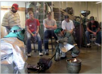
Dr. Sam Ramrattan (facing camera) and an assistant demonstrate pouring liquid metal into a mold. High school students view the process from behind a safety curtain in the Parkview Campus Metal Casting Lab.
