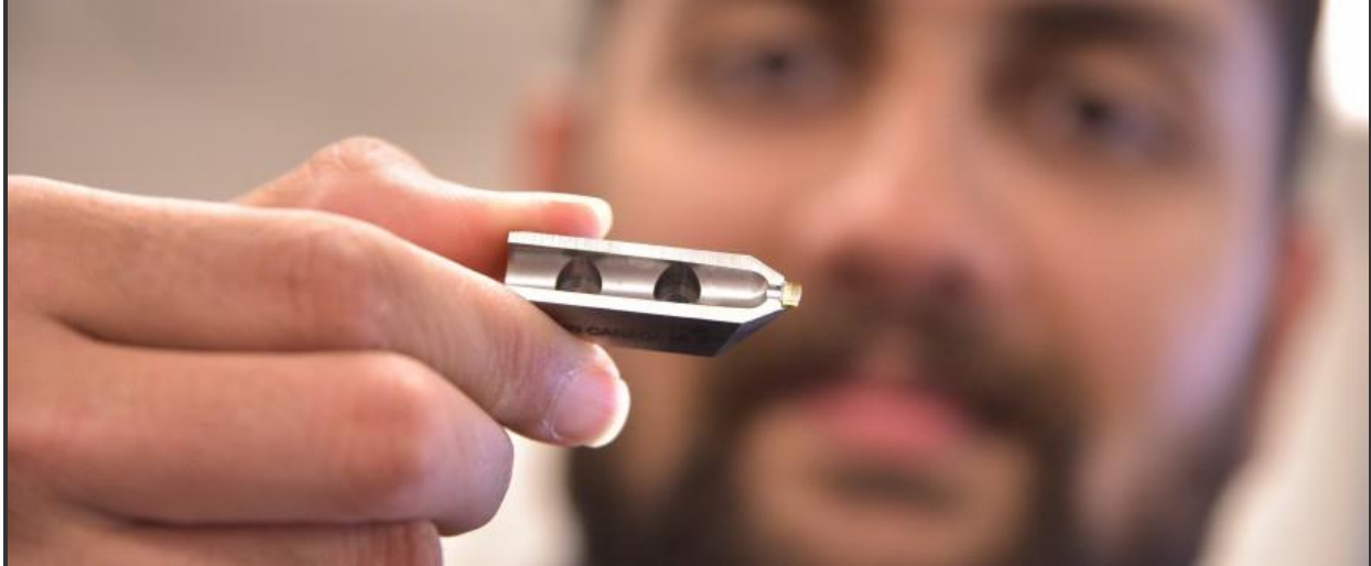
Dr. Deepak Ravindra displays one of Micro-LAM's diamond-cutting tools.
