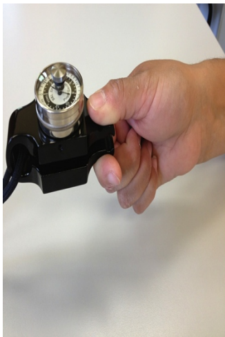
Figure 2. A B&L pinch gauge used for both lateral and 3-jaw chuck trials.
