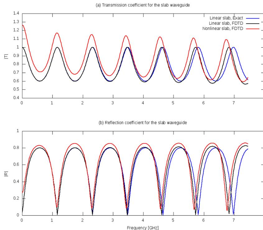
**Fig. 4:** Transmission and reflection spectra for the slab waveguide.
