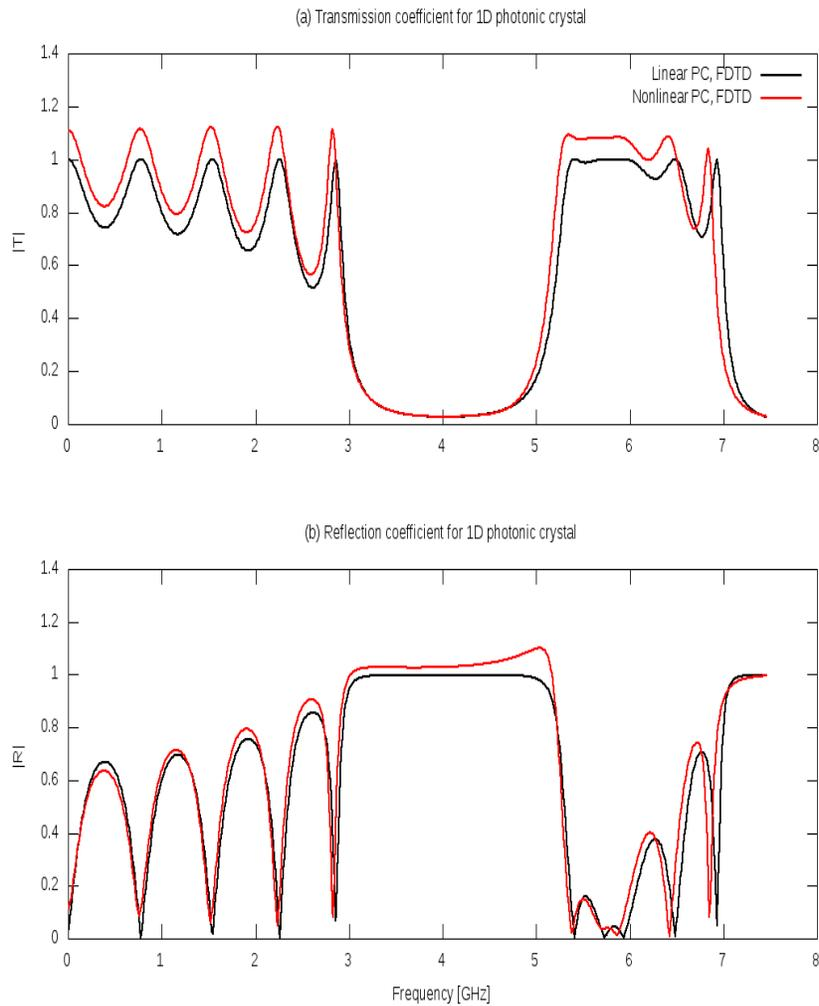
**Fig. 5:** Transmission and reflection spectra for 1D photonic crystal formed with 5 periods.
