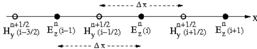
**Fig. 1:** A typical 1D FDTD space chart of the Yee algorithm showing spatial offset between the electric and magnetic fields,  $E_z$  components symbolized as closed circles and  $H_y$  components as open circles on the  $\hat{x}$ -axis (line of computational domain). The direction of Poynting vector is along the positive  $x$ -axis.
