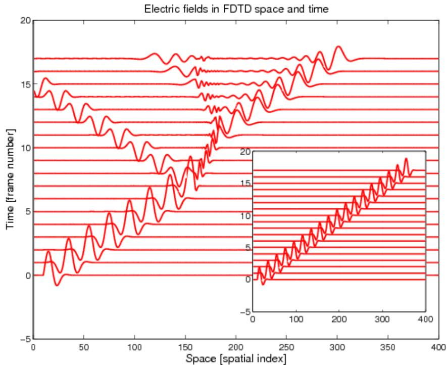
**Fig. 3:** Waterfall plot of the electric field distribution in a computational domain which has a slab waveguide region (starting at node 150 and ending at node 175) with linear dielectric
