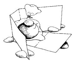
Solar cookers come in three basic categories: box cookers, panel cookers and parabolic cookers but they all operate using the same principle.
