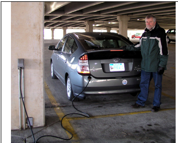
Dr. John Patten plugs in to the electric grid at the CEAS campus to recharge the battery that was added to his Prius. The plug-in unit meter enables him to record volts, amps, watts, kilowatt hours and time. A full charge takes about 3 hrs.
