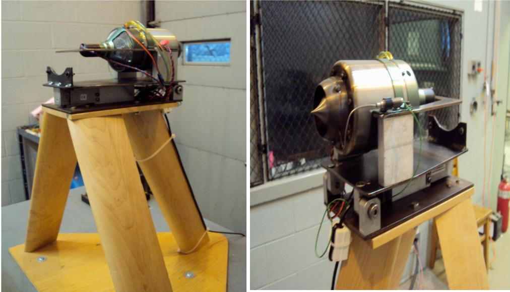
Figure 1. Turbojet engine lab setup
