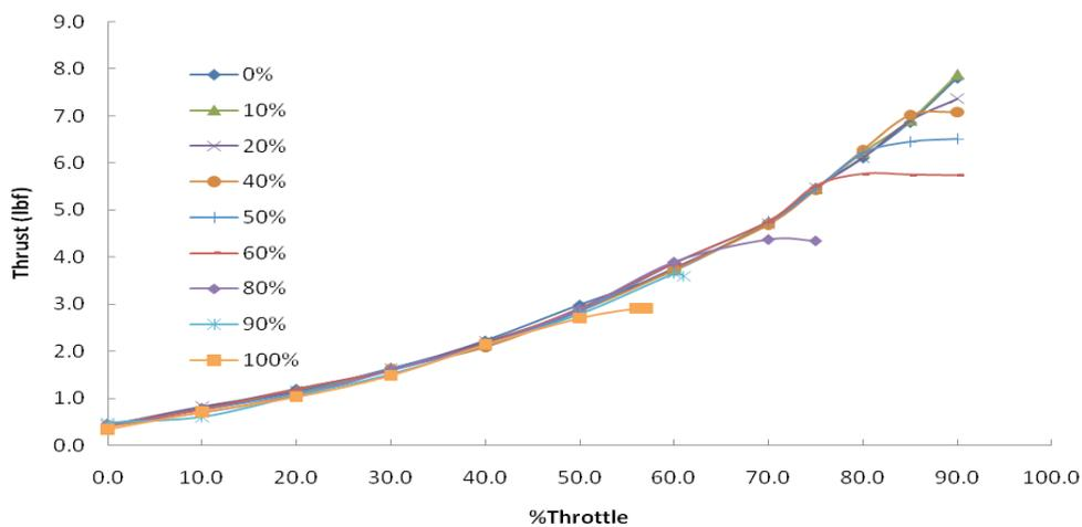
Figure 4. Engine thrust variation with fuel mixing ratio
