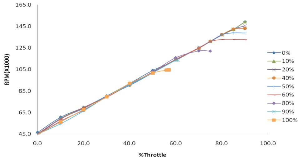
Figure 3. Engine speed variation with the throttle level.
