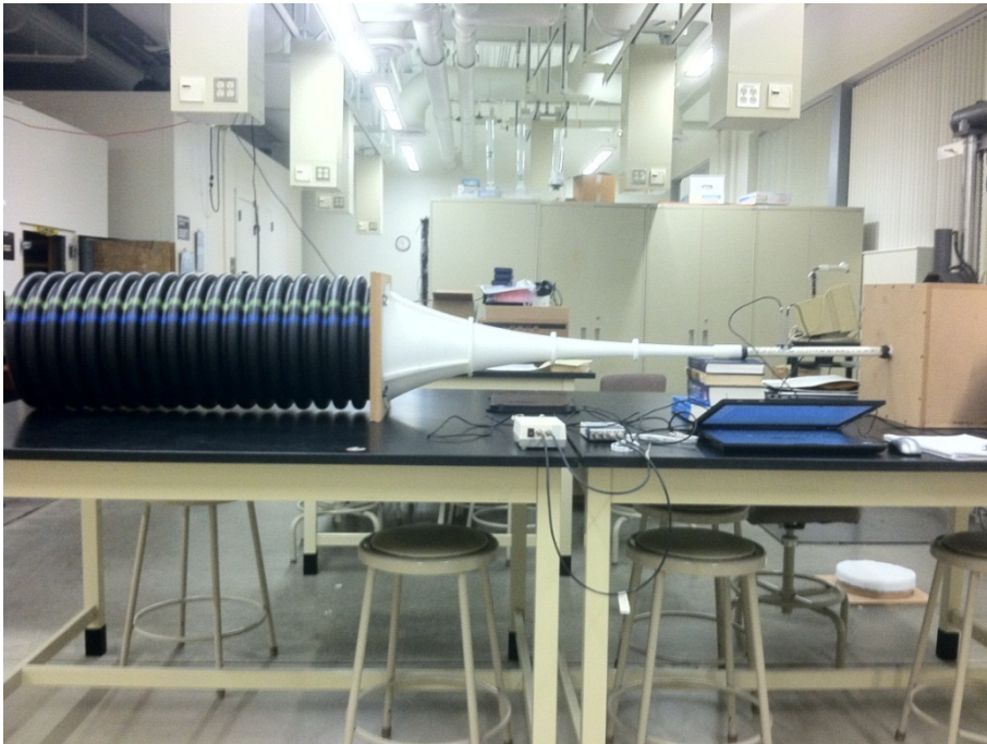
Figure 26 Experimental arrangement with sound source, impedance tube, catenoid, absorbing termination, and data acquisition system
