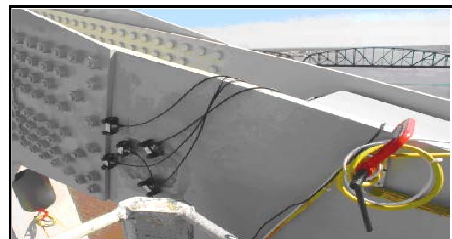
Figure 2. Remote bridge health monitoring for fatigue (Source: Kosnik 2008)
