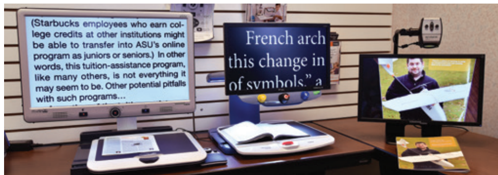
The vision rehabilitation clinic has a range of devices to assist low-vision patients, including closed-circuit television systems that can magnify and even audibly read written material.
