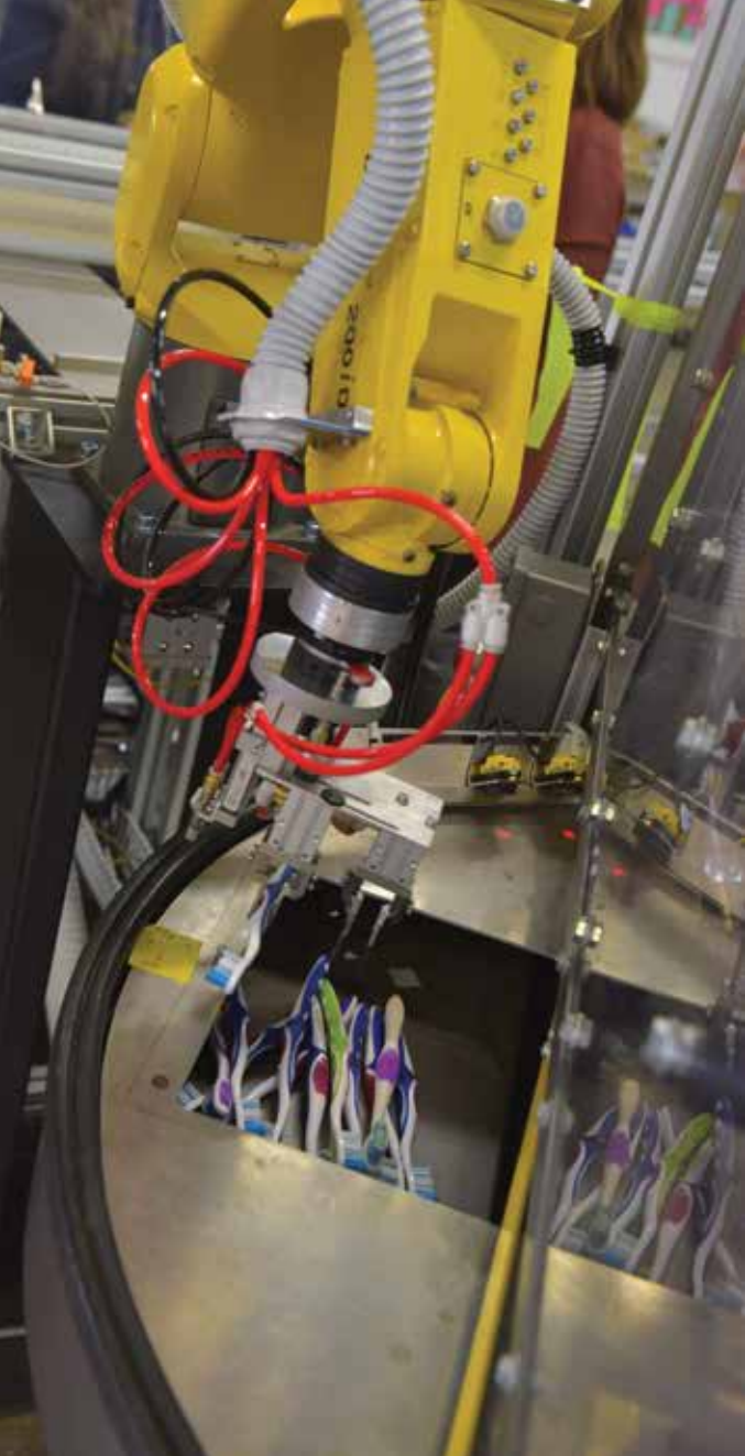
For one of its customers, Singh Automation created a programmable “arm” that feeds toothbrushes into another machine.
