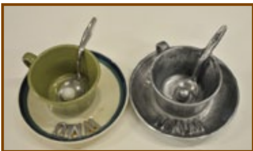
Left is the model design setting and right the casted piece, handmade cast using green sand without cores.
