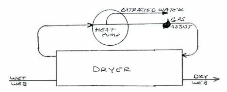
Since the differential temperature is smaller than at  $300^{\circ}$ F (or  $149^{\circ}$ C) it will take a dryer bed (according to test data) 1.6 times as large assuming 10% relative humidity. If all other dimensions are increased by that same factor, then the carrying medium would have to have a volumne of 4800 cf. If it took one minute for the air to pass through the system, then:
