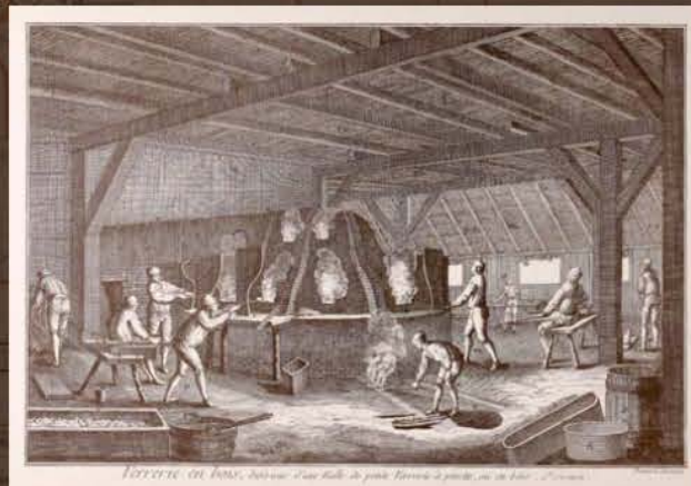
Example of a French glass manufacturer. The image depicts a fundamental component of eighteenth century glass production: a wood-fired furnace, which produced the high temperatures necessary for glass manipulation. Photo courtesy of Denis Diderot and Jean Le Rond d'Alembert's Encyclopédie.
