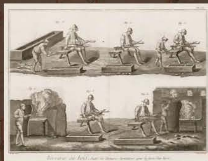
This image, originally taken from Denis Diderot and Jean Le Rond d'Alembert's Encyclopédie, depicts a small-scale glass factory in France. The workers are utilizing a wood-fired furnace to complete the final steps in shaping a goblet.
