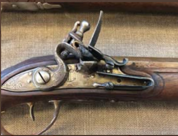
A close-up of the mechanics of a flintlock ignition system. Photo courtesy of Meghan Williams.
