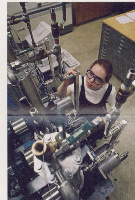
WMU operates one of only a handful of U.S. facilities devoted to tribology, which seeks ways of reducing the damage wear causes in interacting mechanical parts.
