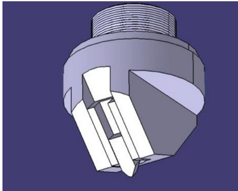
Figure 3. Nozzle that holds the diamond drill bit.
