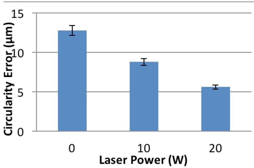
Figure 4. Edge entrances quality compared to an ideal circle (a: without laser, b: 10W, c: 20W, d: after increasing the rigidity of setup)
