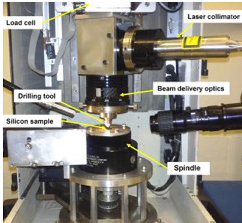
Figure 2.  $\mu$ -LAD Setup used to perform the tests.
