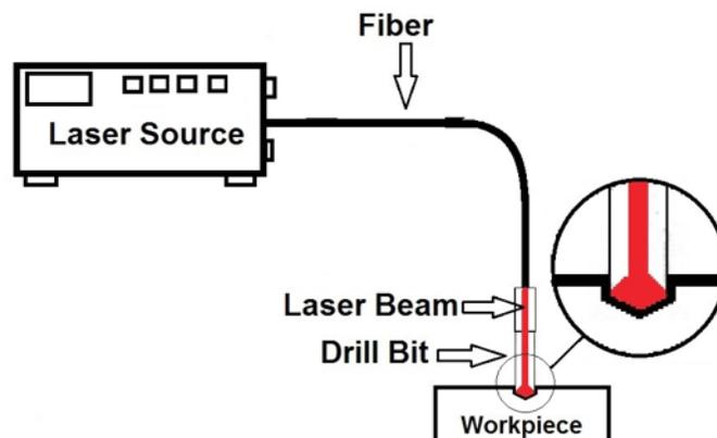
Figure 1. Schematic of  $\mu$ -LAD process
