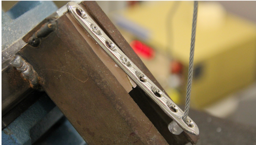
Figure 4.7: Experimental setup for oblique load pullout with cortical bone layer
