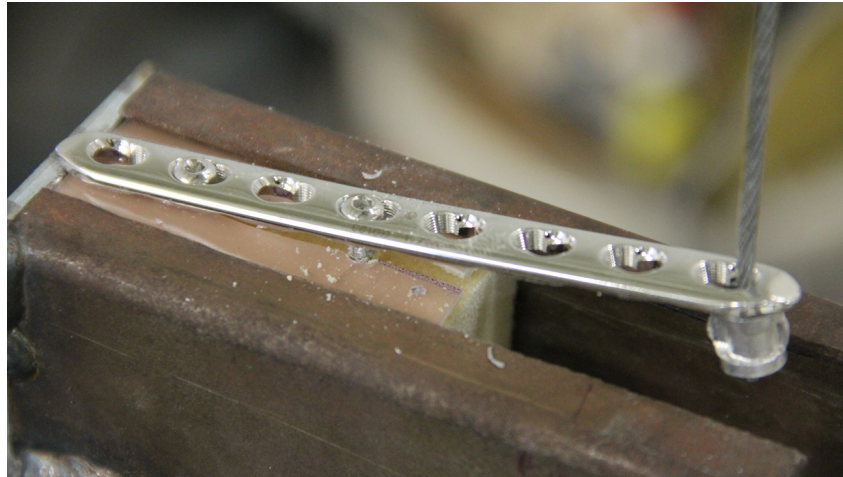
Figure 4.10: Experimental setup for normal load pullout with 1mm thick cortical layer
