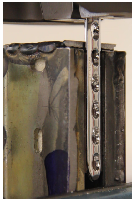
Figure 4.14: Experimental setup for shear load
