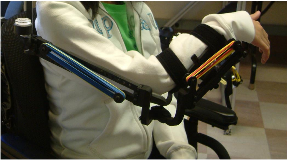
Figure 1. The Wilmington Robotic Exoskeleton (WREX) mounted to a wheelchair.
