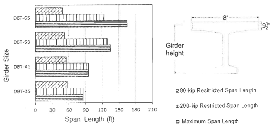
Figure 4. Maximum Applicable and Weight Restricted Span Lengths of DBT with 9.5 in. Thick Flange
