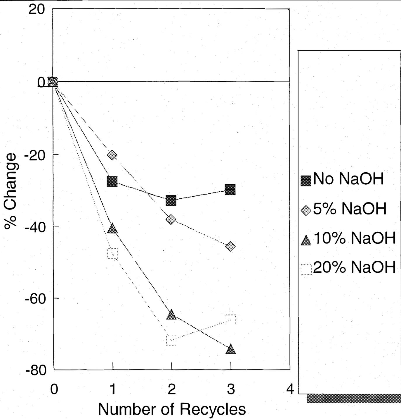
Figure 3. Effect of NaOH Addition on Tensile Index after Successive Recycling (% Change)
