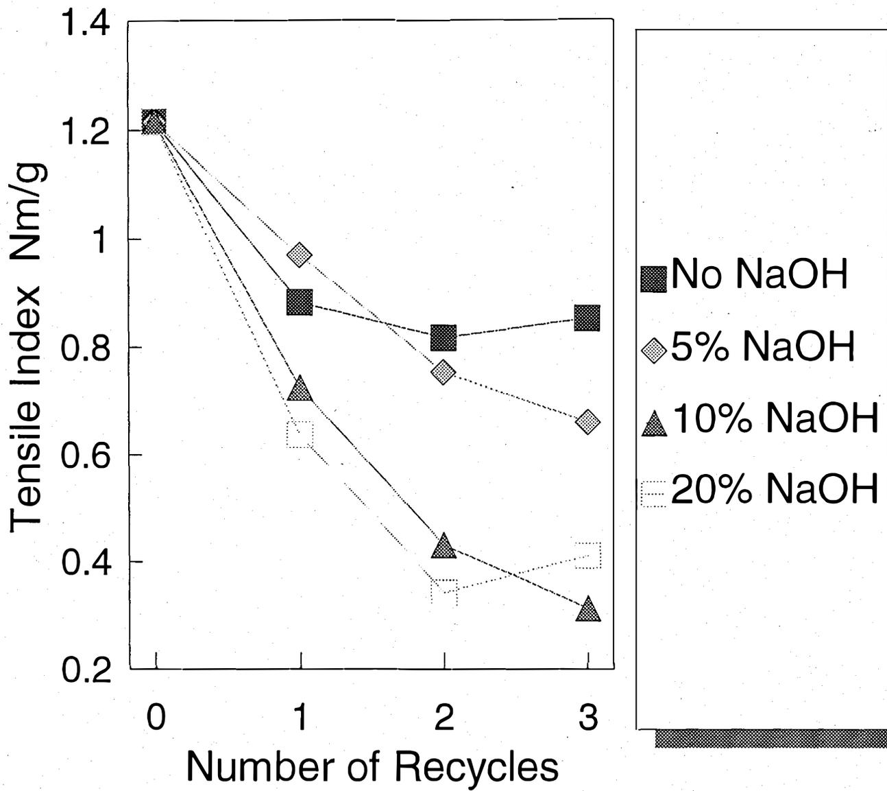
Figure 2. Effect of NaOH Addition on Tensile Index after Successive Recycling
