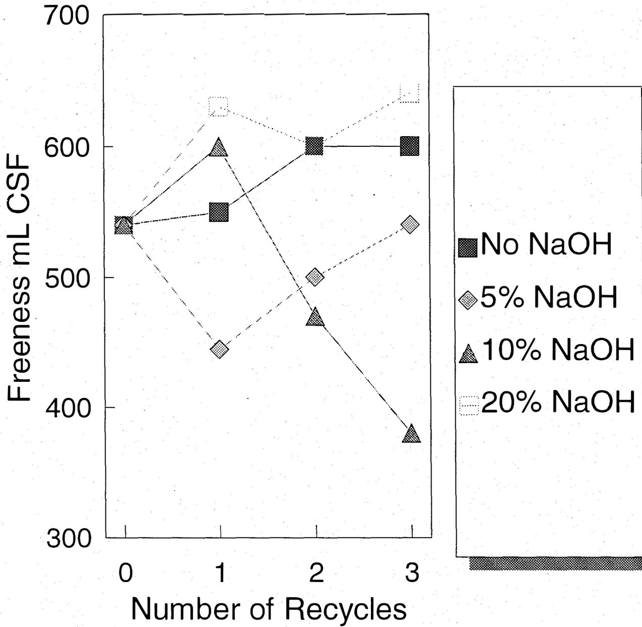
Figure 1. Effect of NaOH Addition on Freeness after Successive Recycling
