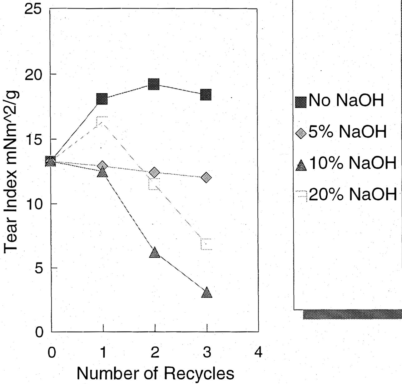
Figure 4. Effect of NaOH Addition on Tear Index after Successive Recycling
