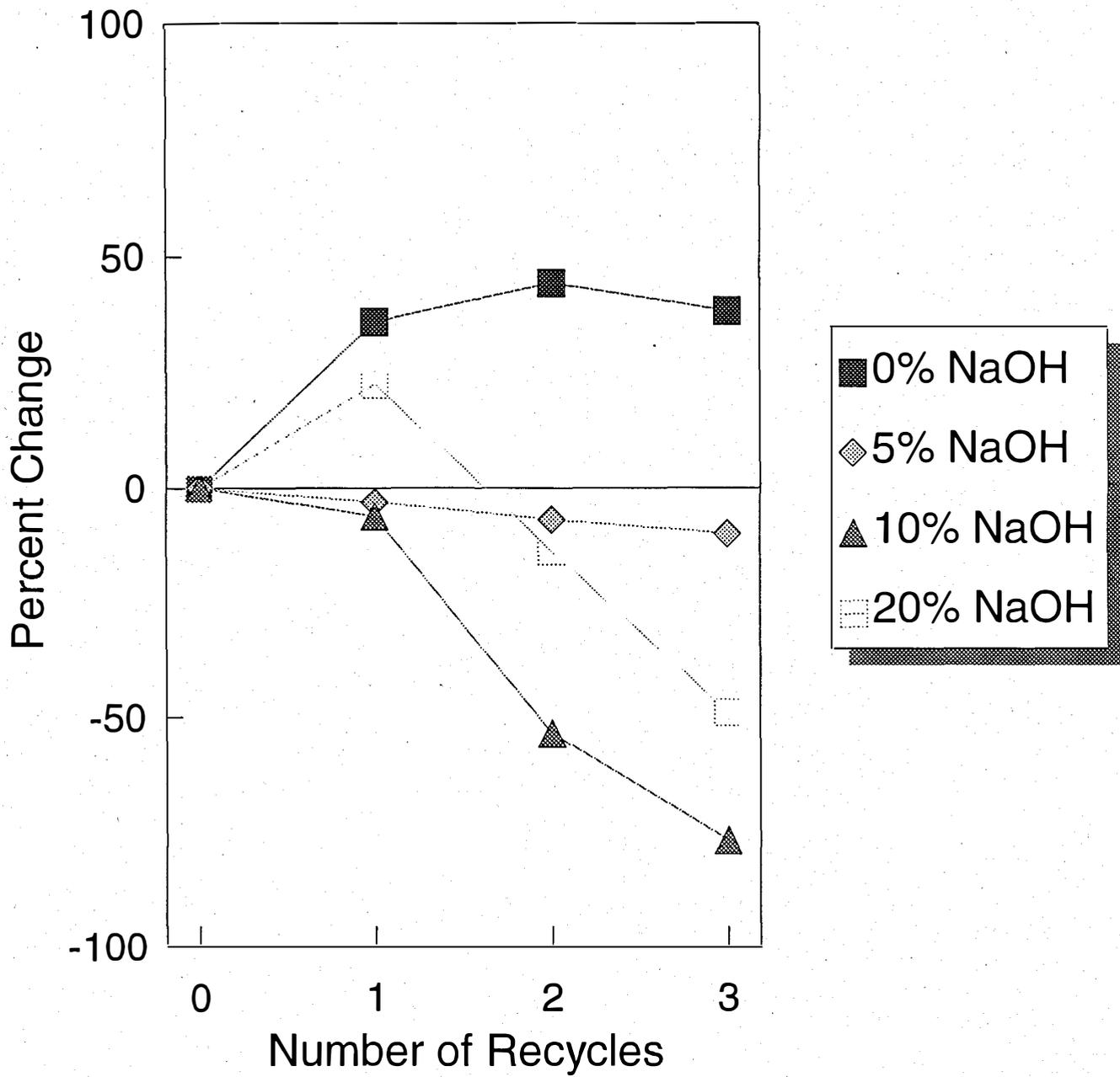
Figure 5. Effect of NaOH Addition on Tear Index after Successive Recycling (% Change)
