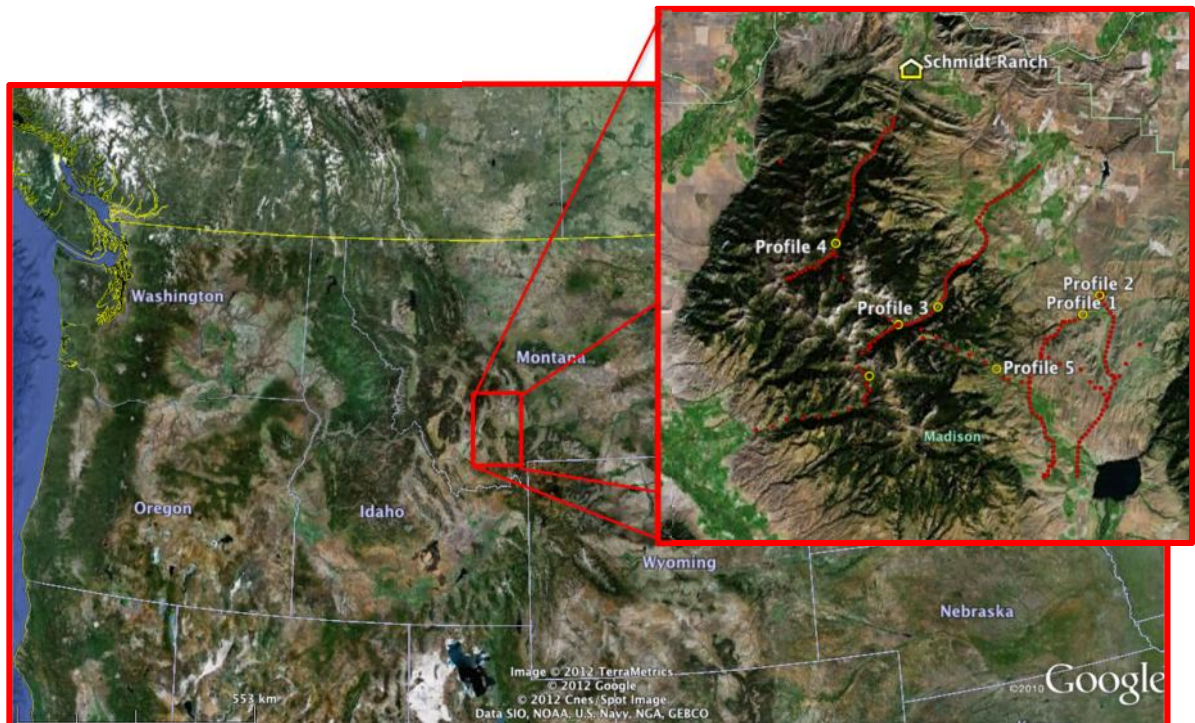
Figure 3: Survey area of the Tobacco Root Mountains over the Tobacco Root Batholith. The dotted red lines indicate each gravity station with yellow circles as base stations for each individual transect.
