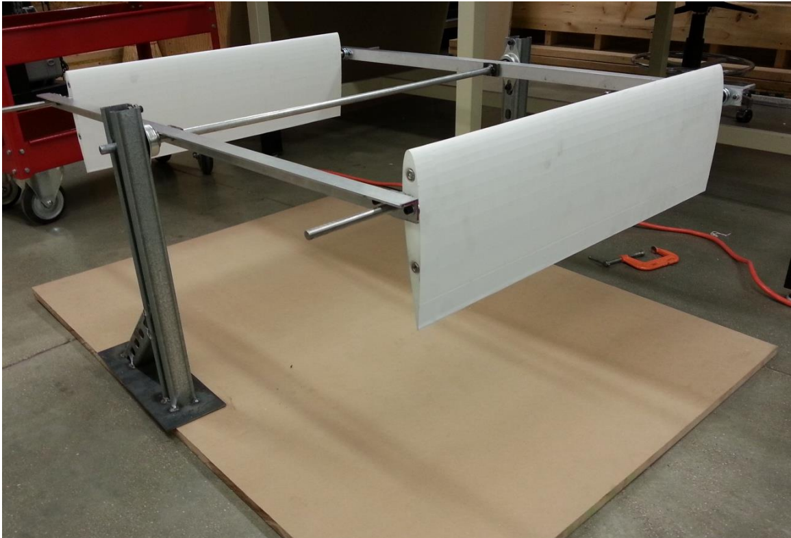
Figure 34: Isometric view of the model oscillator without counter balance.
