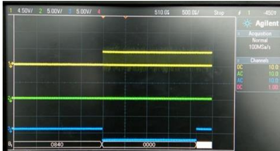
Figure 5-10 Output of the Pattern Generator Board (MSO-X 3034A)
