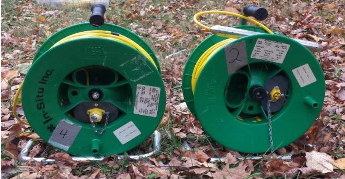
Figure 4-6 In-Situ pressure transducers and their calibration coefficients.
