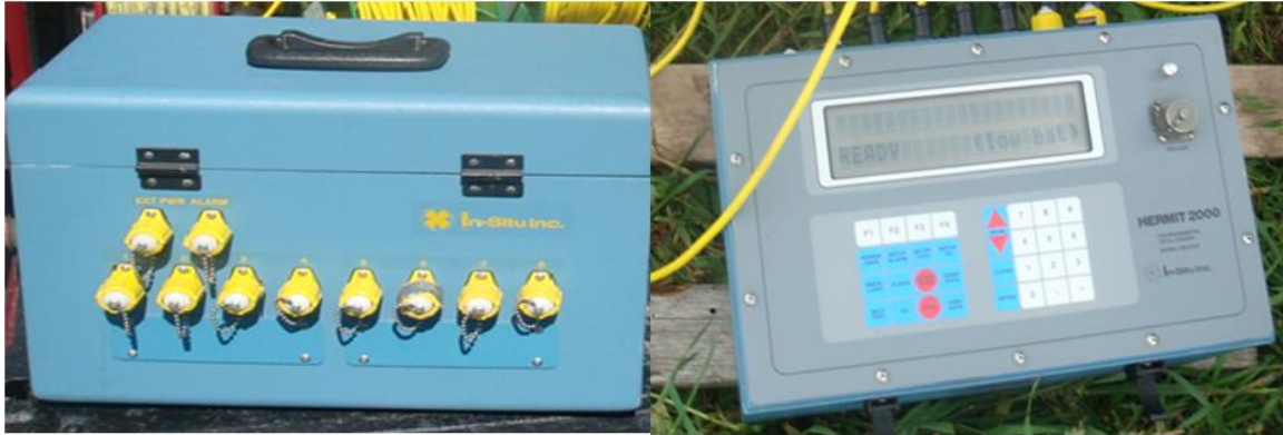
Figure 4-5 Hermit 2000 data logger (from Alfaifi, 2015).
