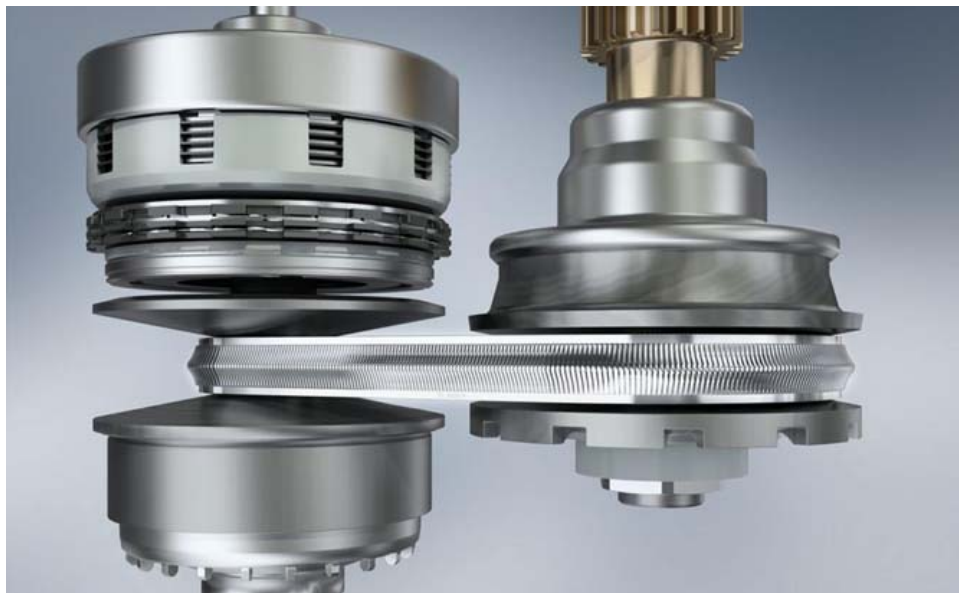
Figure 1: Pulley and belt configuration for a variable diameter CVT [1]
