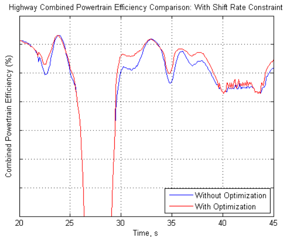
Figure 41: 25-second section of Highway combined powertrain efficiency comparison: CVT shift rate constraint applied.
