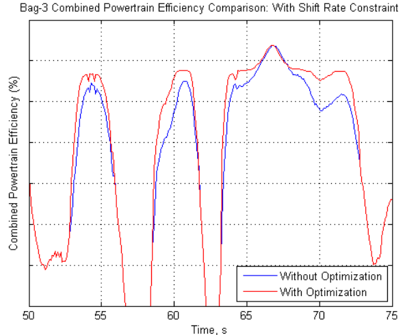
Figure 17: 25-second section of Bag-3 combined powertrain efficiency comparison: CVT shift rate constraint applied.
