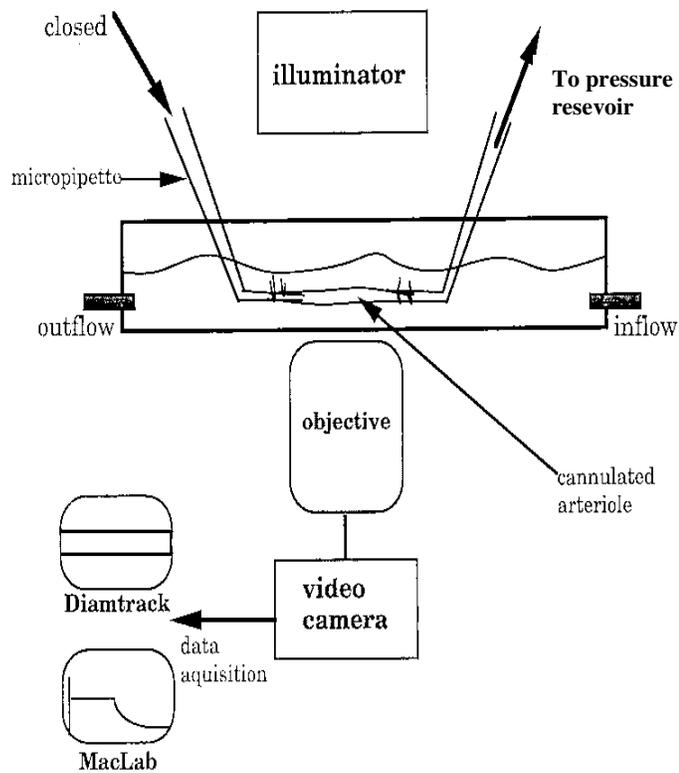
Fig. 5- Cannulated Arteriole Set Up for Experimental Protocols.
