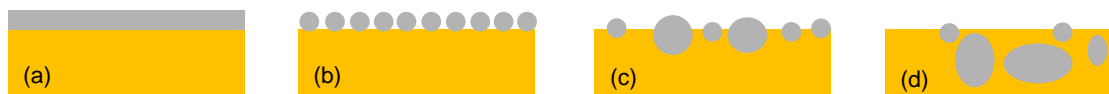
Figure 54. Schematic diagram of (a) Ni thin layer on Si substrate (b) metal nano-particles formation on Si (c) Change in topography, agglomeration and loss of catalytic activity (d) diffusion due to plasma treatment and/or CNT growth process.
