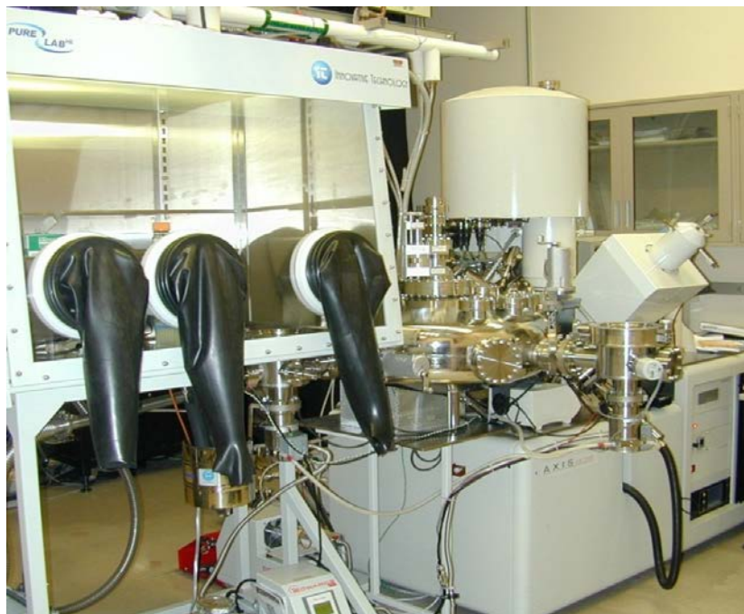
Figure 25. AXIS Ultra DLD XPS system from Kratos Analytical for the x-ray photoelectron spectroscopy measurements of thin films.
