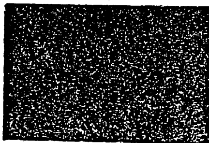
Figure 8. Hologram when the reference beam passes through a fiber optic bundle.
