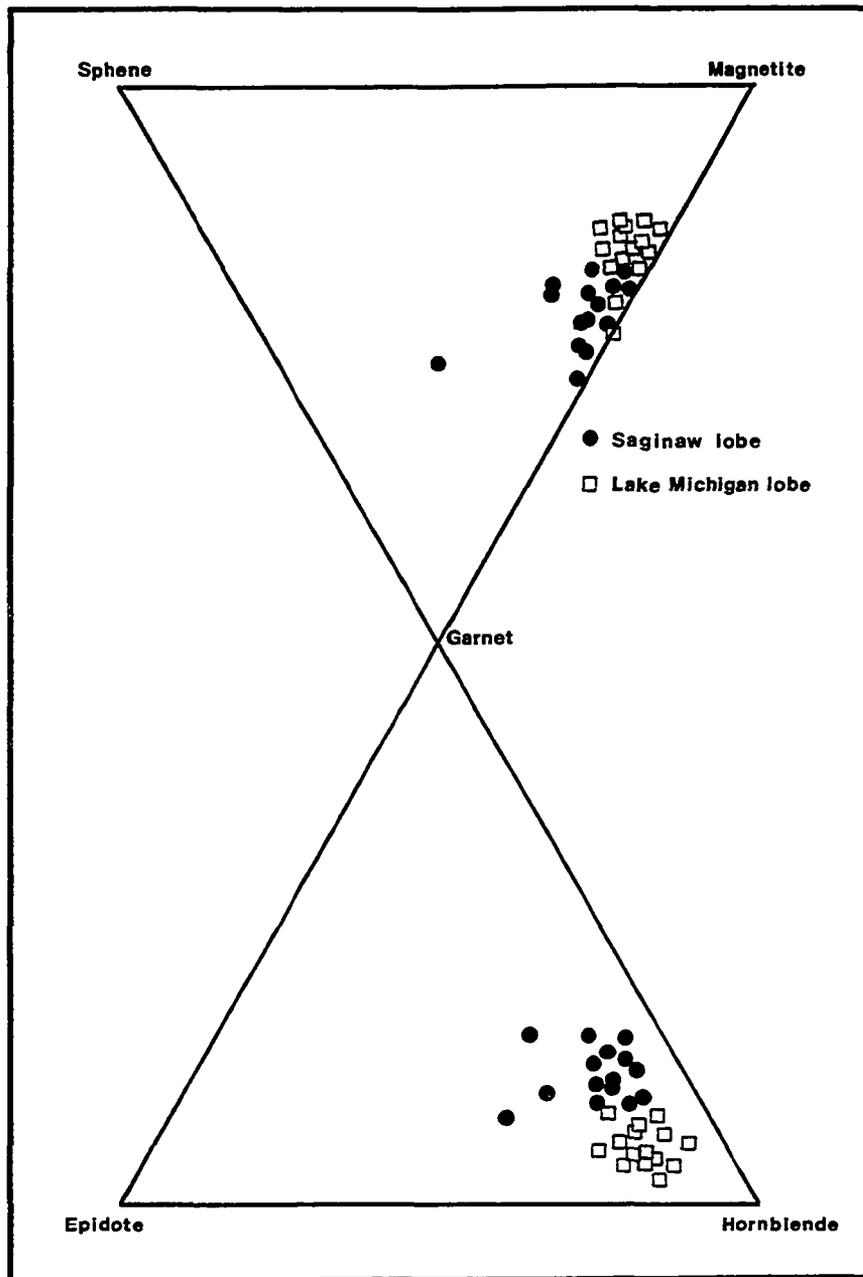
Figure 17. Ternary plots of heavy mineral assemblages occurring in the fine plus very fine (120 + 230 mesh) sand fraction of samples from tills of the Saginaw and Lake Michigan lobes.
