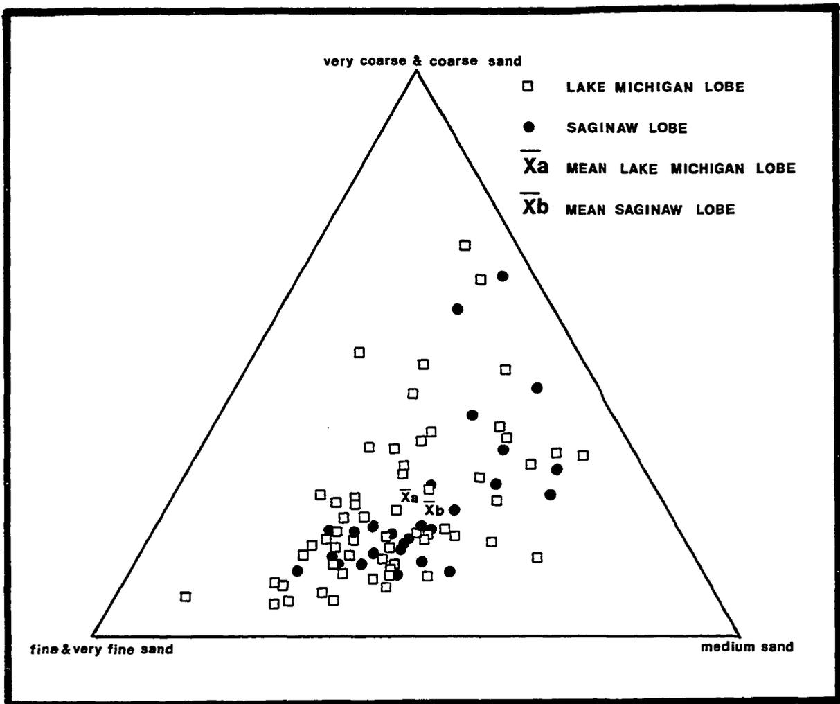
Figure 13. Ternary plot of the very coarse-coarse (18+35 mesh), medium (60 mesh), and fine-very fine (120+230 mesh) sand fractions in samples from both the Lake Michigan and Saginaw lobes showing the mean from each group of samples.
