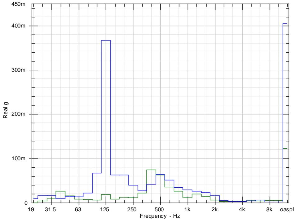
**Figure 34: Comparison of accelerometer readings on the bracket in the X direction, between the speed-increasing (green) and mass modified speed-increasing (blue) motor assemblies [mg].**
