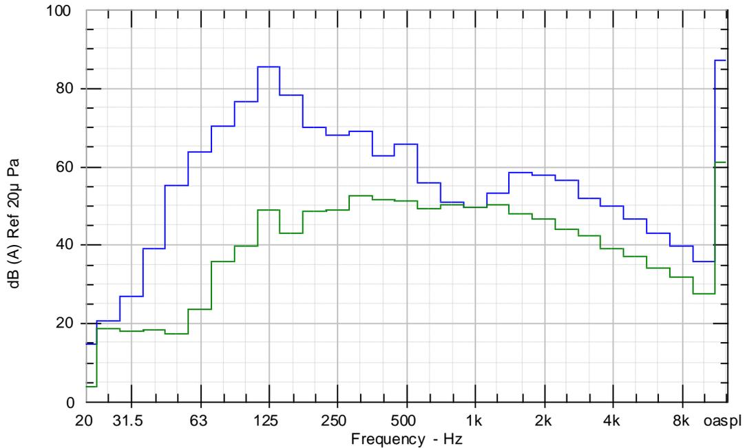
**Figure 23: Comparison of sound pressure levels in the reverberation chamber, between when the dryer was running (green), and when noise was played back at the dryer (blue) [dBA].**
