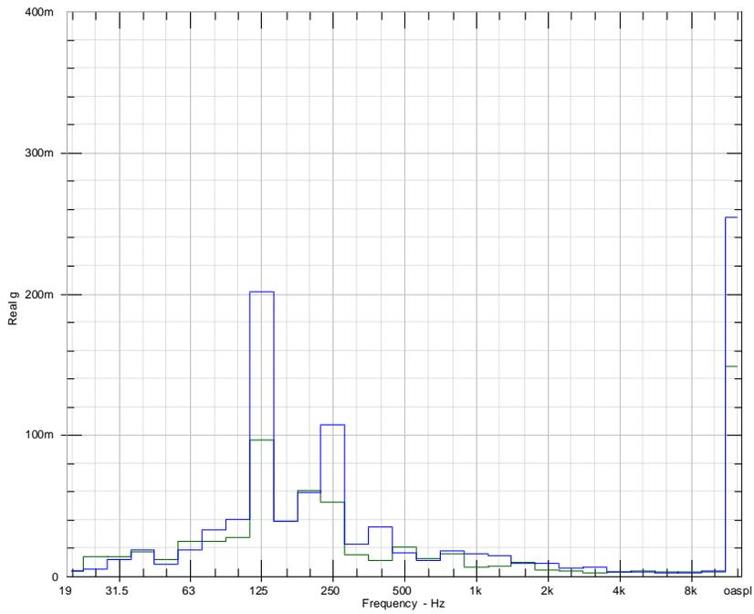
**Figure 40: Comparison of accelerometer readings on the bracket in the Y direction, between the speed-increasing (green) and secondary mass modified speed-increasing (blue) motor assemblies [mg].**
