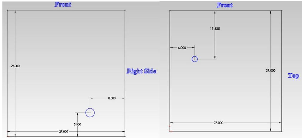
**Figure 75: Dimensions of Base Accelerometer Placement, Left, and Wall accelerometer Placement, right.**
