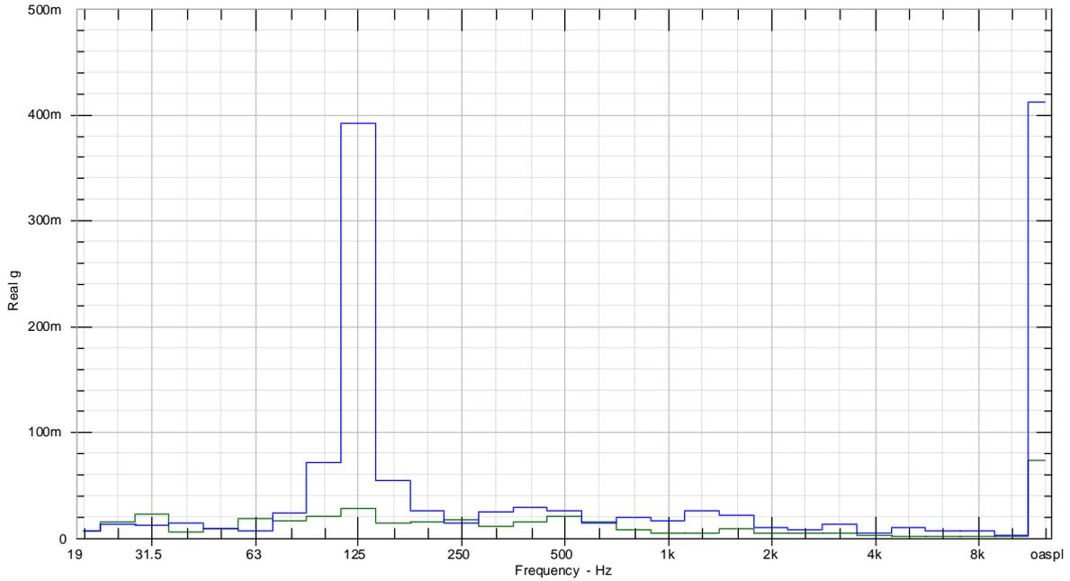
**Figure 19: Comparison of accelerometer measurements on the base of the cabinet, between the standard (green) and speed-increasing (blue) motors [mg].**
