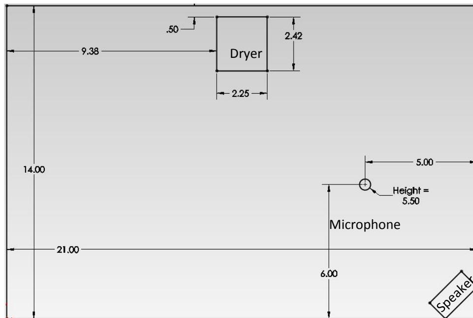
**Figure 77: Layout of Reverberation Chamber (\*note: Dimensions are in ft.)**
