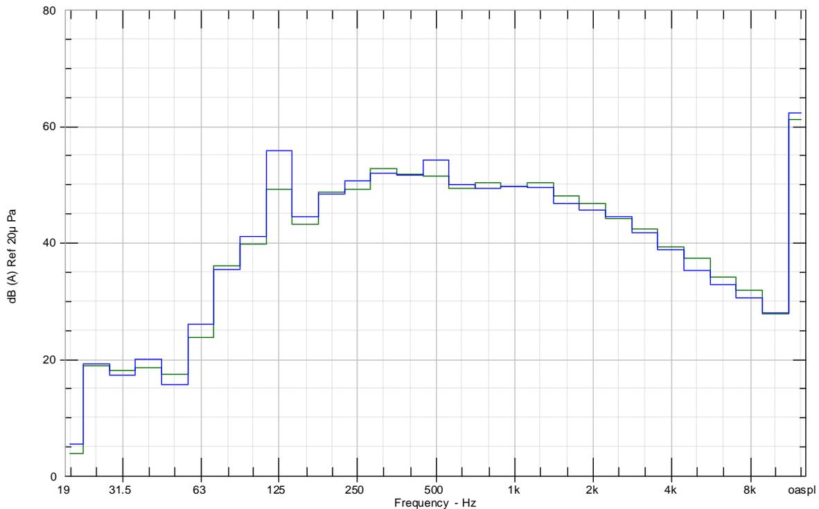
Figure 33: Comparison of sound pressure levels in the reverberation, between the speed-increasing (green) and mass modified speed-increasing (blue) motor assemblies [dBA].
