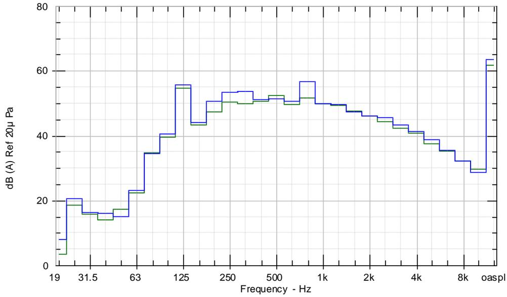
Figure 54: Comparison of sound pressure levels in the reverberation chamber, between speed-increasing (green) and secondary bracket modified speed-increasing motor assemblies [mg].
