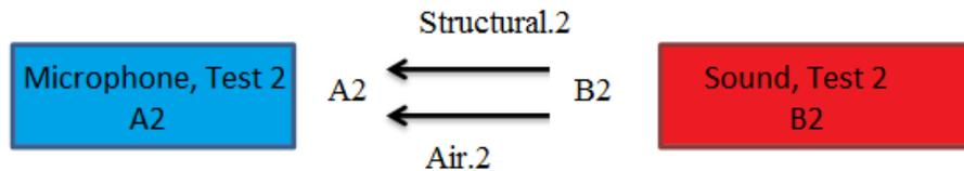
By subtracting test 1 from test 2, a relationship between the structural contributions can be isolated. The assumption is made that the *airborne* components of both tests are equal.
