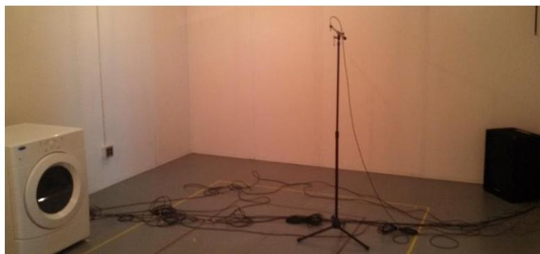
Figure 15: WMU testing setup, showing the location of the dryer and single microphone.
