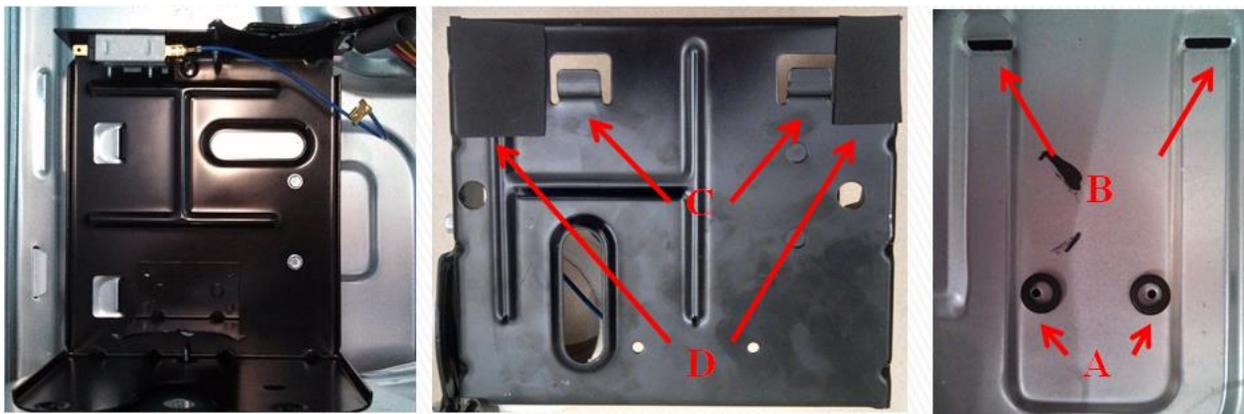
Figure 31: Bracket modifications, including rubber grommets and foam insulation.
