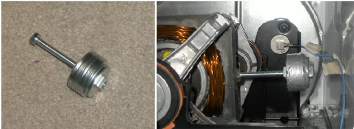
Figure 32: A tuned absorber for 125 Hz, individually, left, and attached to the motor, right.
