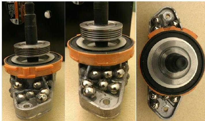
Figure 28: Initial weight addition of 67g to the speed-increasing attachment with side vies, left & center, and top view, right.
