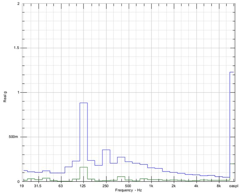
**Figure 39: Comparison of accelerometer readings on the motor, between speed-increasing (green) and secondary mass modified speed-increasing (blue) motor assemblies [mg].**
