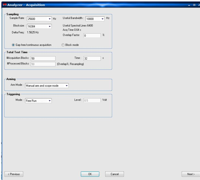
**Figure 81: Acquisition Setup**
