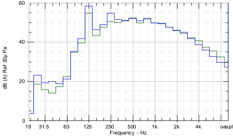
**Figure 41: Comparison of sound pressure levels in the reverberation chamber, between speed-increasing (green) and bracket modified speed-increasing (blue) motor assemblies [dBA].**
