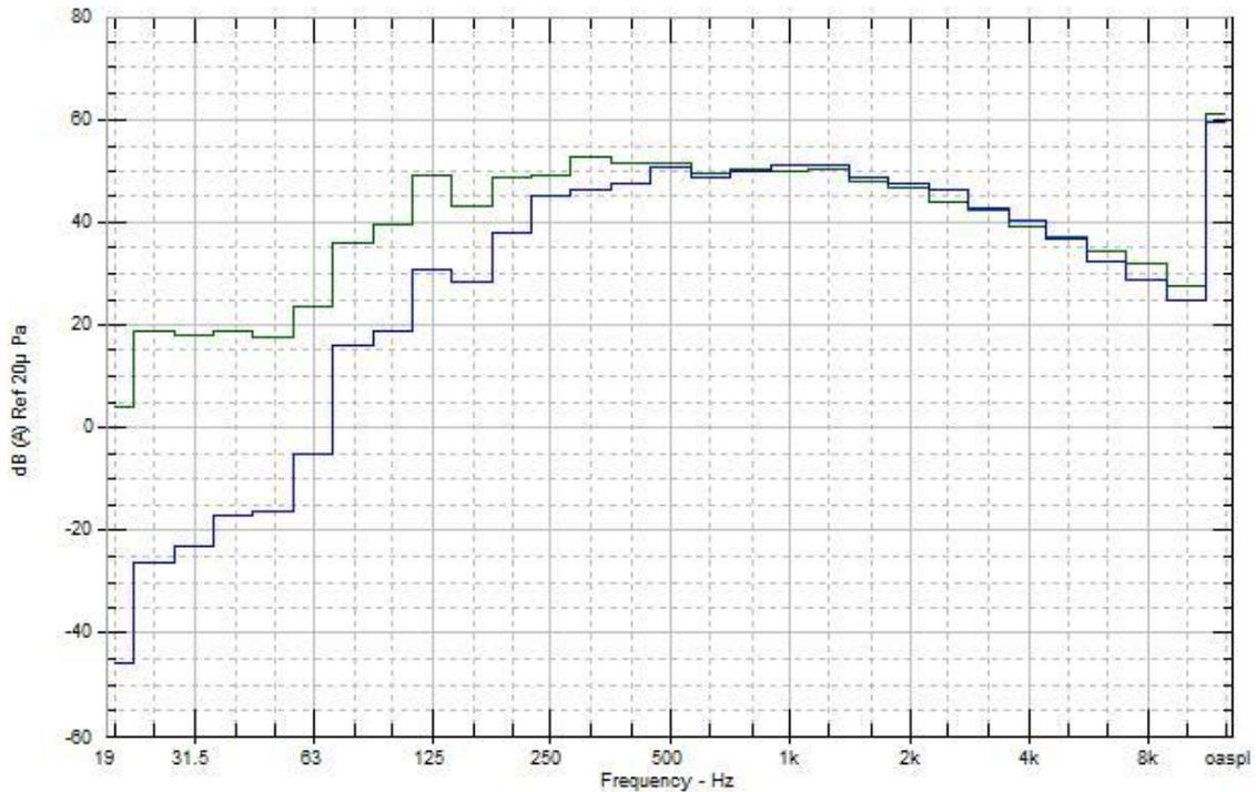
**Figure 36: Comparison of sound pressure levels in the reverberation chamber, between speed-increasing (green) and secondary mass modified speed-increasing (blue) motor assemblies [dBA].**
