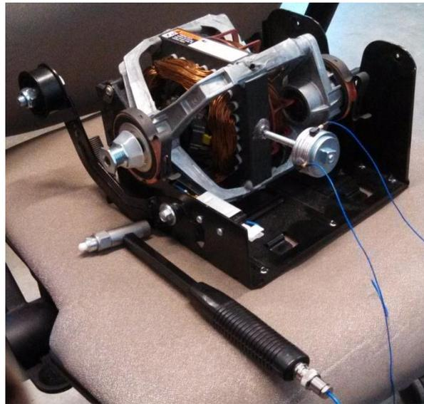
Figure 62: Setup for impact hammer testing.
