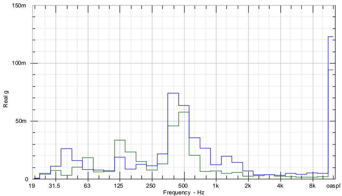
**Figure 20: Comparison of accelerometer measurements on the bracket in the X direction, between the standard (green) and speed-increasing (blue) motors [mg].**
