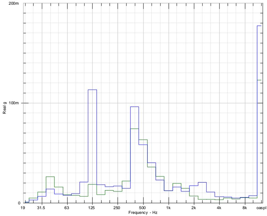
**Figure 37: Comparison of accelerometer readings on the bracket in the X direction, between speed-increasing (green) and secondary mass modified speed-increasing (blue) motor assemblies [mg].**
