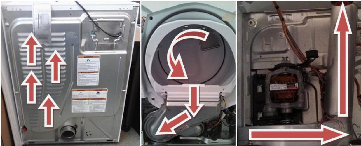
Figure 4: Airflow path through the dryer.
