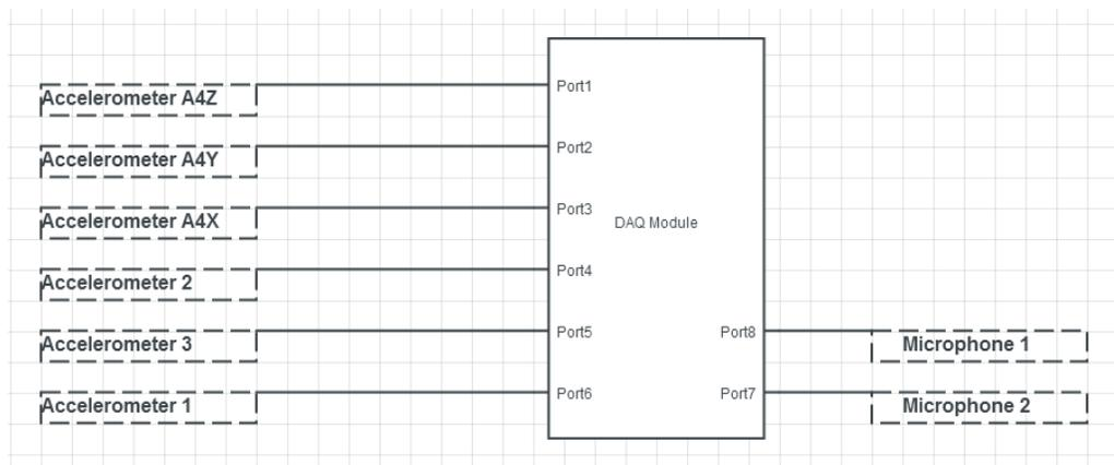
**Figure 74: DAQ Module Connections**
