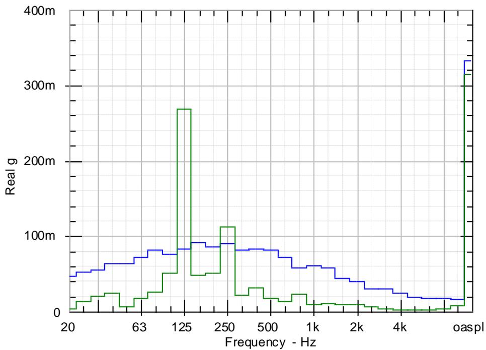
Figure 61: Comparison of accelerometer readings on the bracket in the Z direction, between the speed-increasing (green) and the speed-increasing with secondary tuned absorber (blue) motor assemblies [mg].
