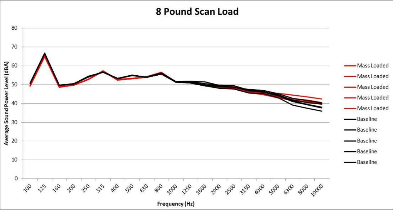
Figure 68: Final Whirlpool testing results for an 8lb Scan Load with the mass corrected motor.
