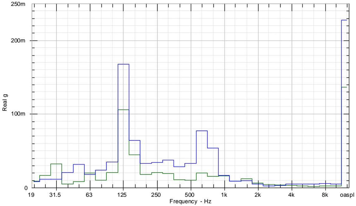
**Figure 21: Comparison of accelerometer measurements on the bracket in the Y direction, between the standard (green) and speed-increasing (blue) motors [mg].**
