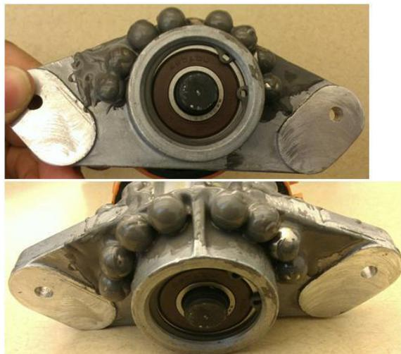
Figure 29: Secondary weight addition with a total weight addition of 115g.
