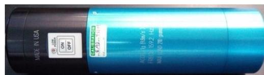
Figure 73: Accelerometer Calibrator
