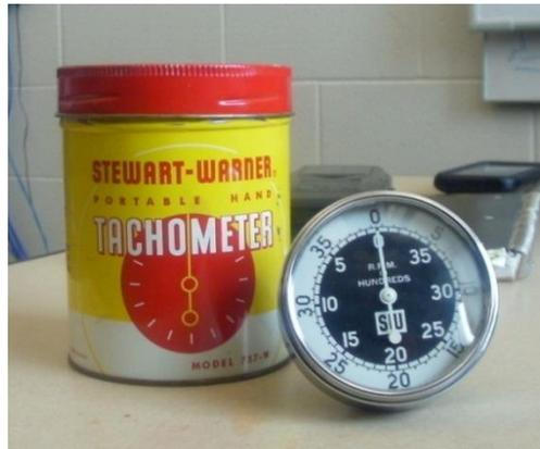
Figure 30: Tachometer used for pulley power loss testing
