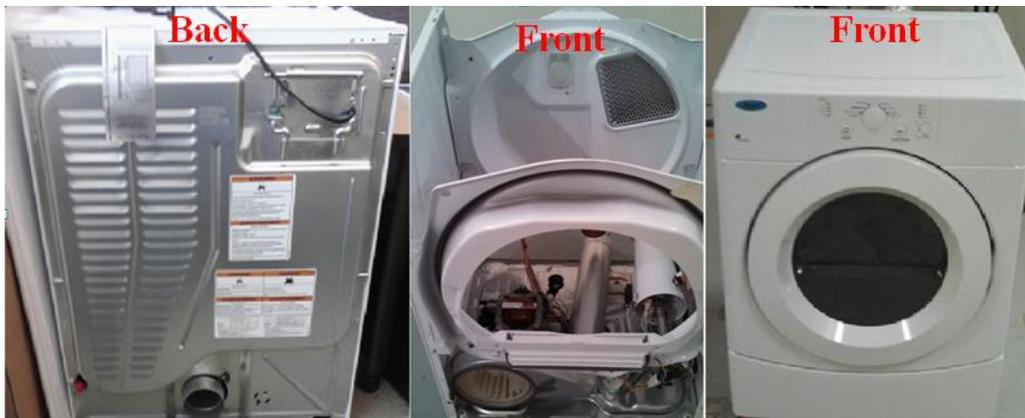
Figure 7: The cabinet system includes the four walls shown, and the top.
