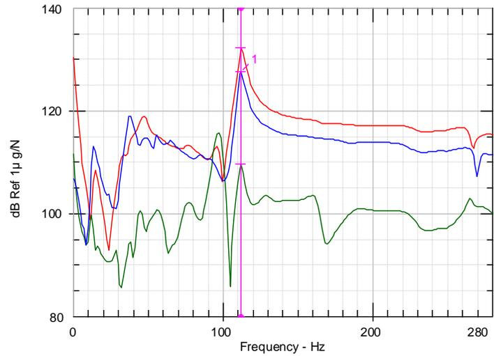
**Figure 64: Side mounted accelerometer results from impact hammer testing for top strike (blue), side strike (green), and angled strike (red).**
