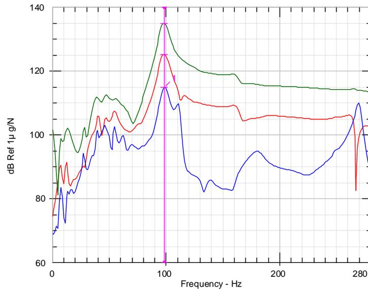
**Figure 65: Top mounted accelerometer results from impact hammer testing for top strike (blue), side strike (green), and angled strike (red).**
