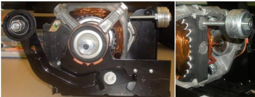
Figure 49: Modified position of tuned absorber
