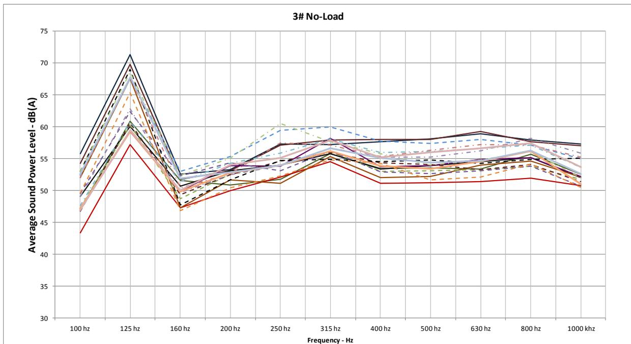
Figure 11: Comparison of different Whirlpool test runs with a 3lb no-load scenario, measuring average sound power level in dBA with the speed-increasing motor.
