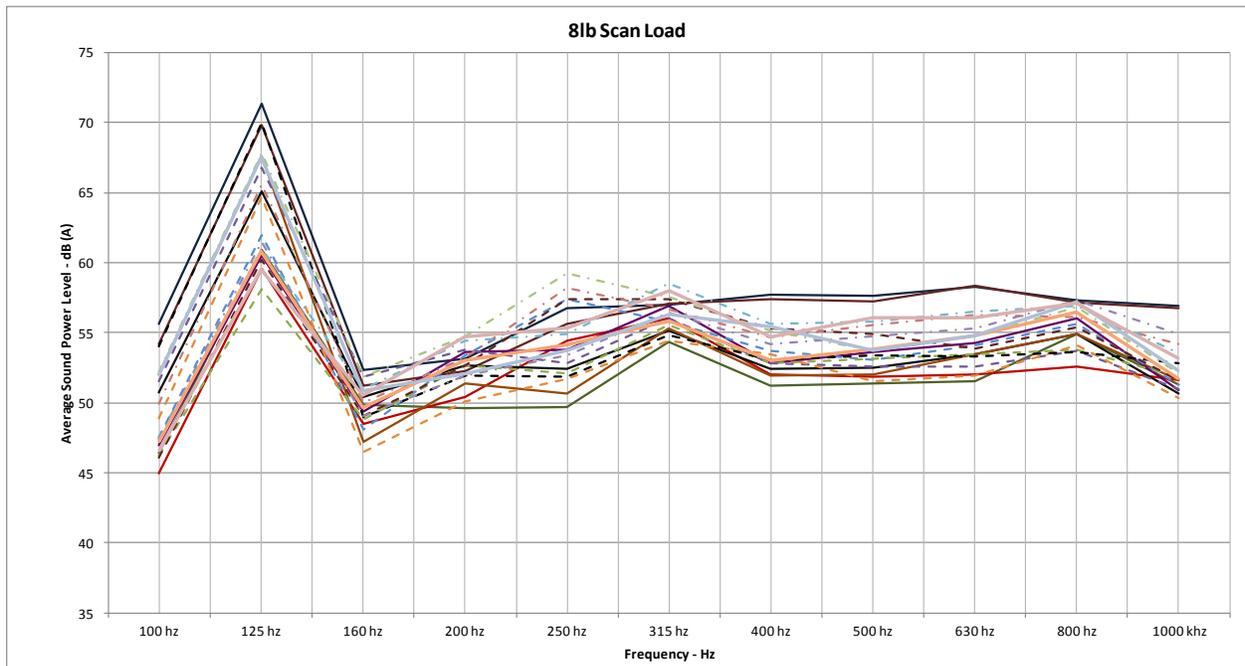
**Figure 12: Comparison of different Whirlpool testing runs with an 8lb scan load, measuring average sound power level in dBA with the speed-increasing motor assembly.**
