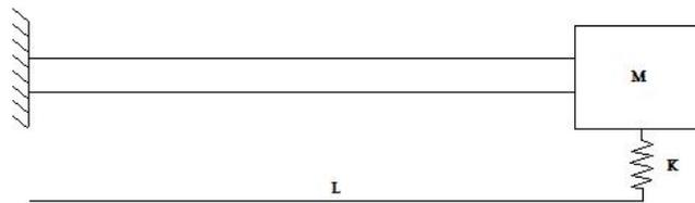
Figure 27: A diagram of a cantilever beam with a point mass and spring.
