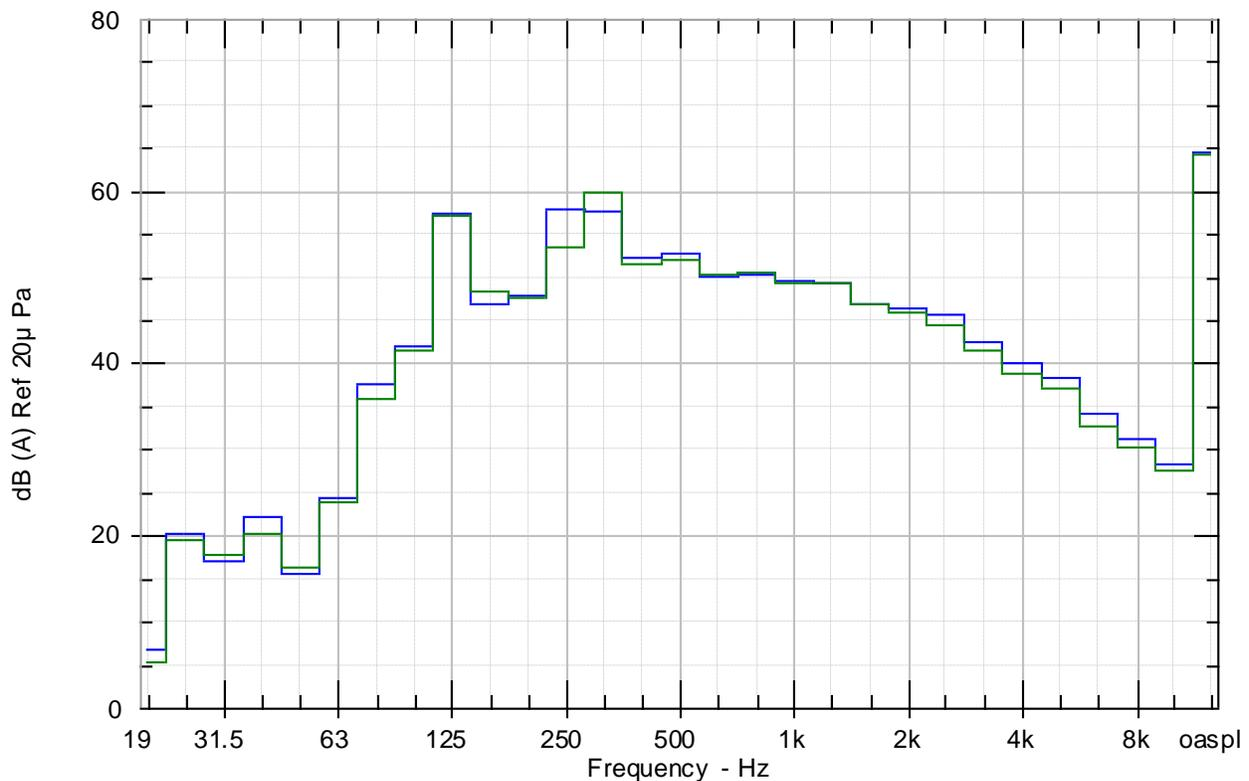
Figure 44: Comparison of sound pressure levels in the reverberation chamber, between speed-increasing (green) and the speed-increasing with tuned absorber (blue) motor assemblies [dBA].
