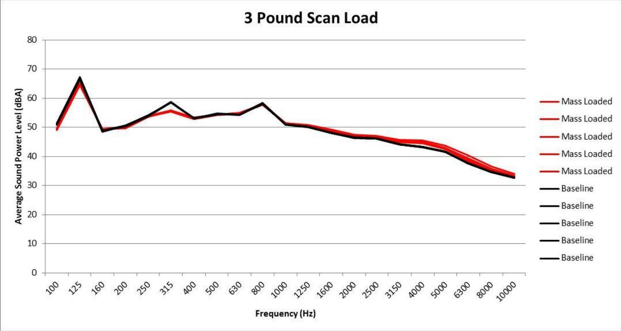
Figure 67: Final Whirlpool testing results for a 3lb No Load with the mass corrected motor.
