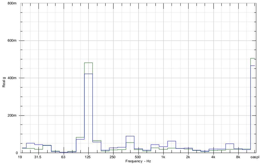
**Figure 51: Comparison of accelerometer measurements on the motor, between speed-increasing (green) and mass corrected speed-increasing (blue) motor assemblies [mg].**
