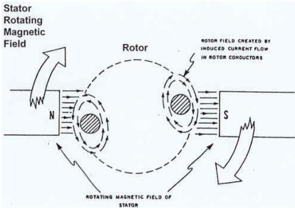
Figure 3: An illustration of the magnetic fields inside an AC induction motor.
