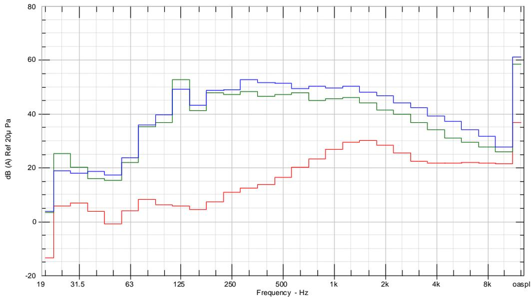
**Figure 17: Comparison of sound pressure levels in the reverberation chamber, between standard (green) and speed-increasing (blue) motors, and background noise (red) [dBA].**
