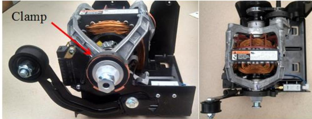
Figure 6: The motor system from the rear, left, and from the top, right, consisting of the motor, its casing, the shaft, and the bracket.
