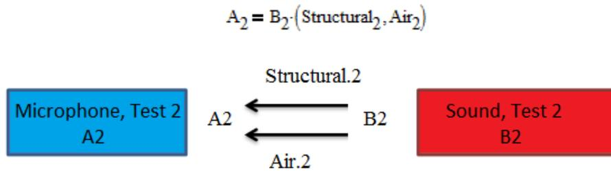
By subtracting test 1 from test 2, a relationship between the structural contributions can be isolated. The assumption is made that the *structural* components of both tests are equal.
