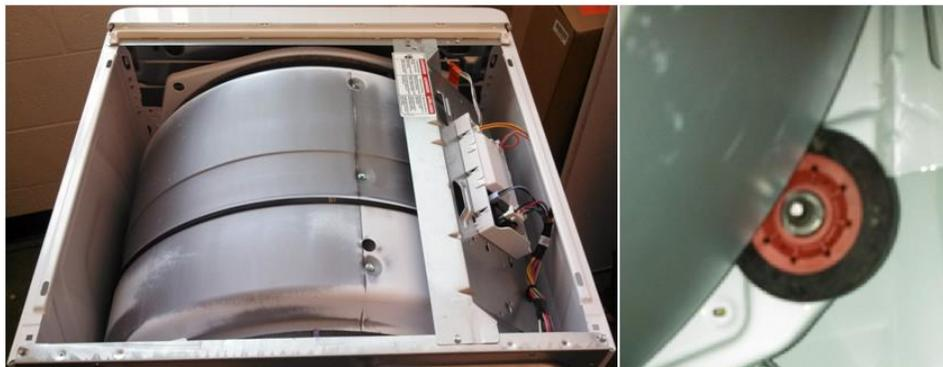
Figure 9: Drum system, including the drum, left, and roller wheels, right.
