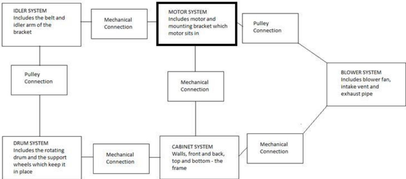
Figure 5: A macro-product map showing the dryer's systems and the connections between them, highlighting the motor system.
