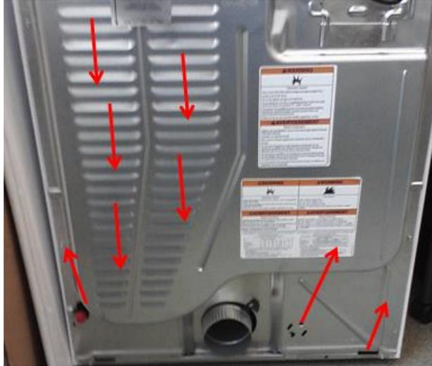
Figure 24: Illustration of airborne noise pathways on the back panel of the dryer.
