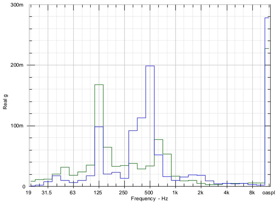
**Figure 35: Comparison of accelerometer readings on the motor in the Y direction, between the speed-increasing (green) and mass modified speed-increasing (blue) motor assemblies [mg].**
