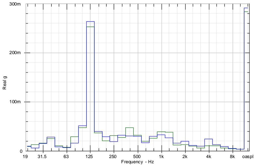
Figure 55: Comparison of accelerometer readings on the base, between the speed-increasing (green) and bracket modified speed-increasing (blue) motor assemblies [mg].
