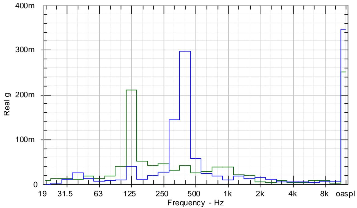
Figure 43: Comparison of accelerometer readings from the bracket in the Y direction, between speed-increasing (green) and bracket modified speed-increasing (blue) motor assemblies [mg].
