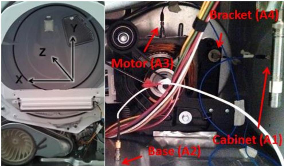
Figure 14: Accelerometer coordinate system, left, and accelerometer placement, right.
