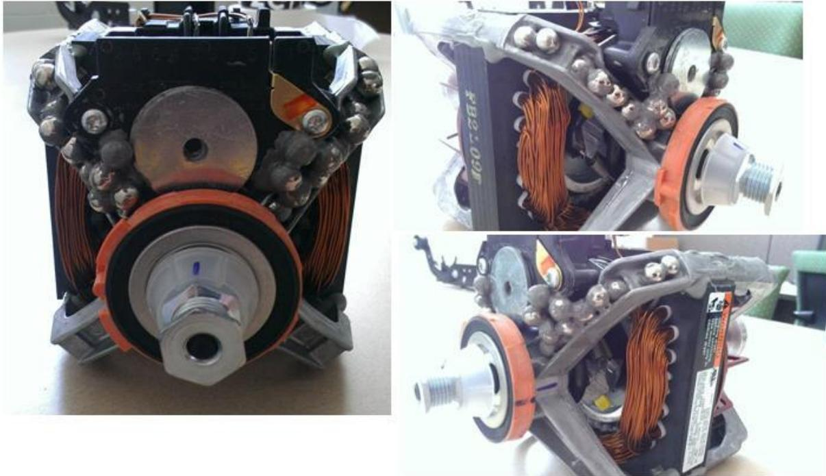
Figure 47: Mass modification on the opposite side of the speed-increasing motor to counteract the weight of the attachment, shown from the front and from either side.
