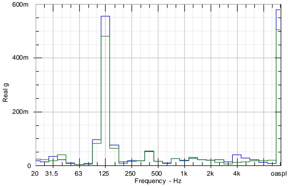
Figure 58: Comparison of accelerometer measurements the motor, between the speed-increasing (blue) and the speed-increasing with secondary tuned absorber (blue) motor assemblies [mg].
