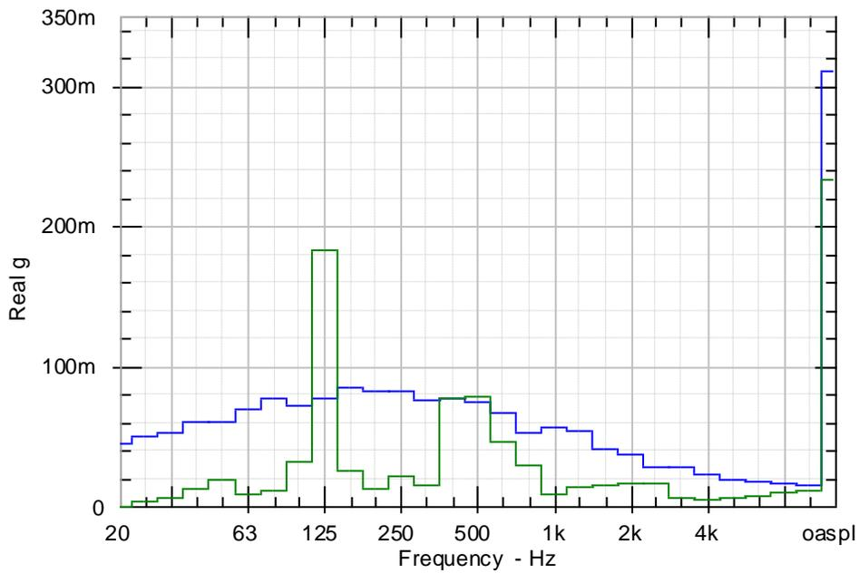
Figure 59: Comparison of accelerometer readings on the bracket in the X direction, between the speed-increasing (green) and the speed-increasing with secondary tuned absorber (blue) motor assemblies [mg].
