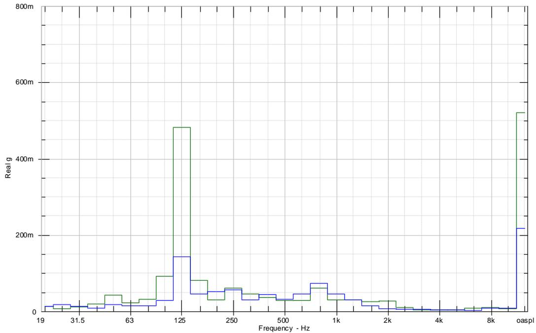
**Figure 53: Comparison of accelerometer measurements on the bracket in the Y direction, between speed-increasing (green) and mass corrected speed-increasing (blue) motor assemblies [mg].**
