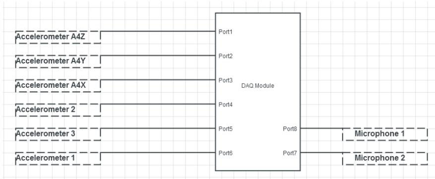
**Figure 16: DAQ wiring schematic.**
