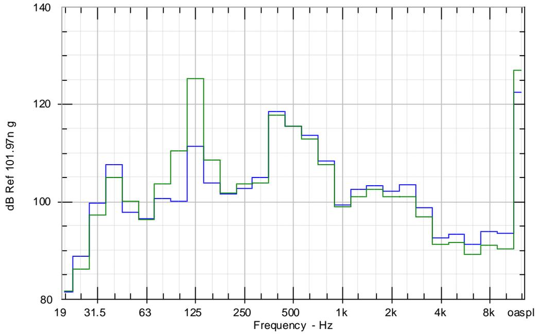
Figure 45: Comparison of accelerometer readings on the bracket in the X-direction, between the speed-increasing (green) and the speed-increasing with tuned absorber (blue) motor assemblies [mg].
