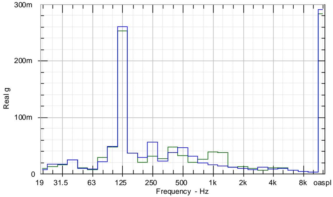
Figure 42: Comparison of accelerometer readings on the base, between speed-increasing (green) and bracket modified speed-increasing (blue) motor assemblies [mg].
