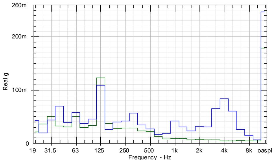
**Figure 18: Comparison of accelerometer measurements on the wall of the cabinet, between the standard (green) and speed-increasing (blue) motors [mg].**
