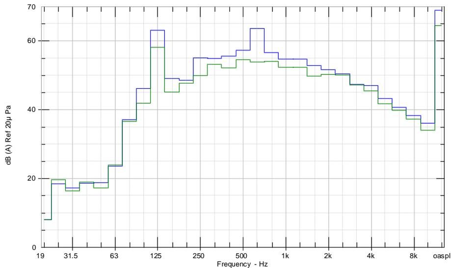
Figure 57: Comparison of sound pressure levels in the reverberation chamber, between the speed-increasing (green) and the speed-increasing with secondary tuned absorber (blue) motor assemblies [dBA].
