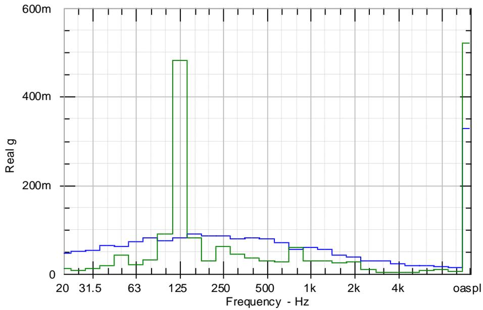
Figure 60: Comparison of accelerometer readings on the bracket in the Y direction, between the speed-increasing (green) and the speed-increasing with secondary tuned absorber (blue) motor assemblies [mg].
