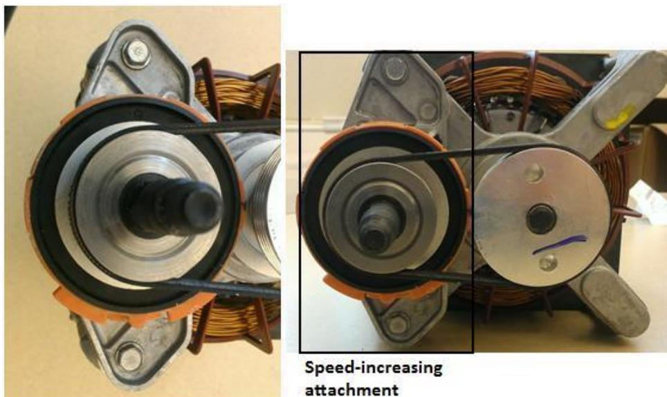
**Figure 25: The speed-increasing attachment required to increase the speed of the blower fan.**
