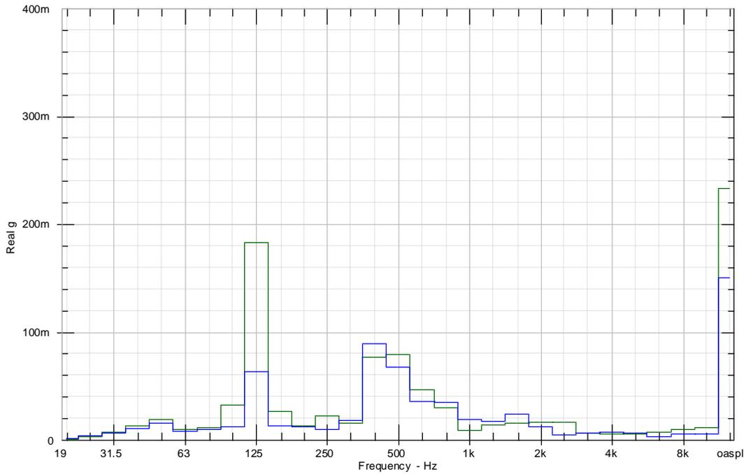
**Figure 52: Comparison of accelerometer measurements on the bracket in the X direction, between speed-increasing (green) and mass corrected speed-increasing (blue) motor assemblies [mg].**
