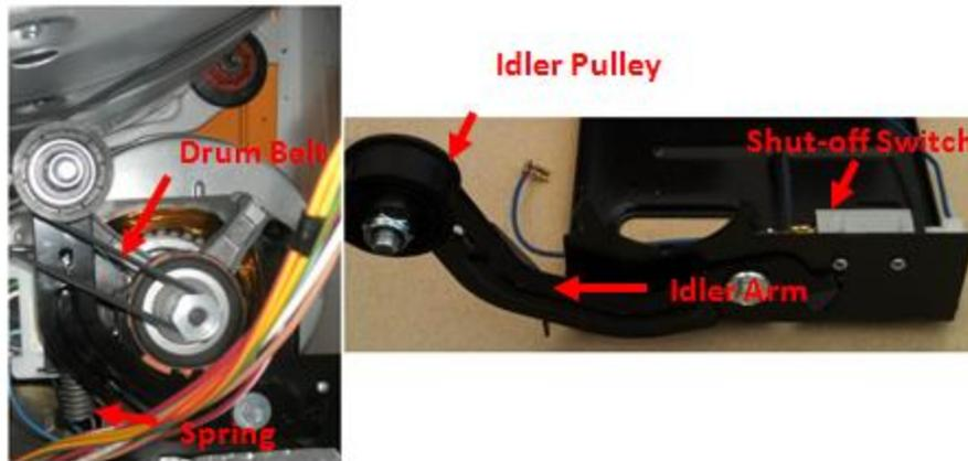
Figure 10: System, including the idler arm, idler pulley, spring, drum belt, and shut-off switch.
