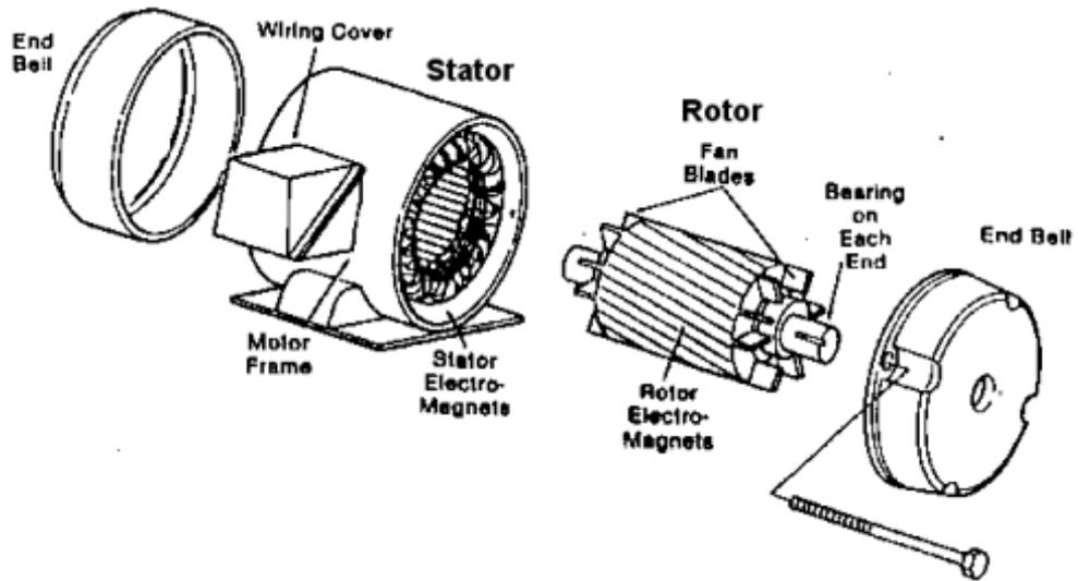
Figure 2: Basic construction of an AC Induction Motor
