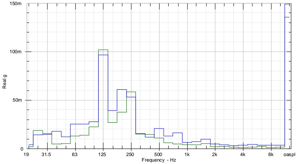
**Figure 22: Comparison of accelerometer measurements on the bracket in the Z direction, between standard (green) and speed-increasing (blue) motors [mg].**
