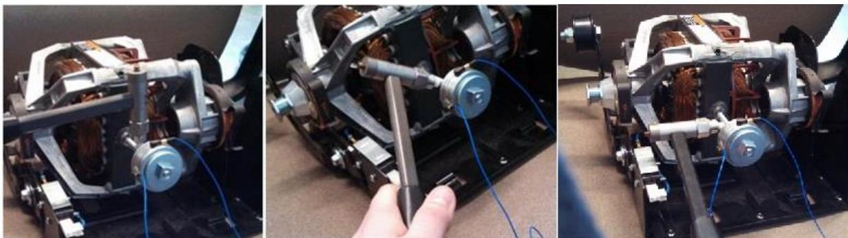
Figure 63: Setup for impact hammer testing, top strike, left, and angled strike, right.
