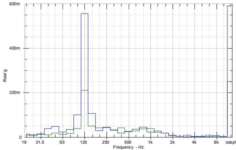
Figure 56: Comparison of accelerometer readings on the bracket in the Y direction, between speed-increasing (green) and secondary bracket modified speed-increasing (blue) motor assemblies [mg].
