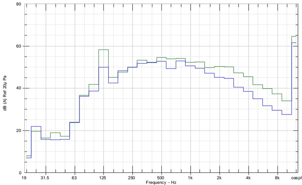
Figure 50: Comparison of sound pressure levels in the reverberation chamber, between speed-increasing (green) and mass corrected speed-increasing (blue) motor assemblies [dBA].
