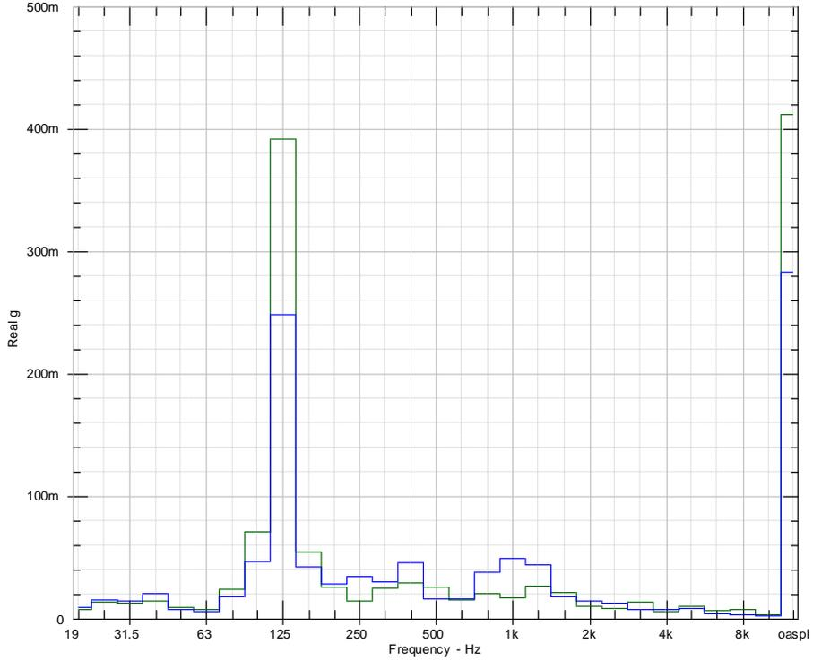
**Figure 38: Comparison of accelerometer readings on the base, between the speed-increasing (green) and secondary mass modified speed-increasing (blue) motor assemblies [mg].**
