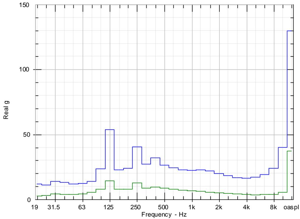
Figure 46: Comparison of accelerometer readings on the motor, between speed-increasing (green) and the speed-increasing with tuned absorber (blue) motor assemblies [mg].
